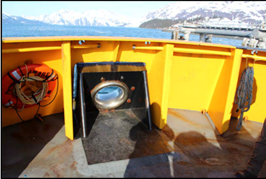
Figure D.7 - Detail of the forward fairlead through which the towline is led for any escort work.
