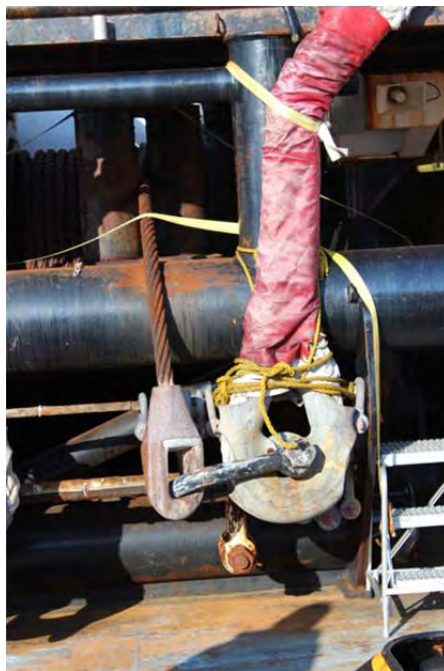
Figure D.3 - Detail of shackled connection between the steel wire on the drum and the ETP system above.
