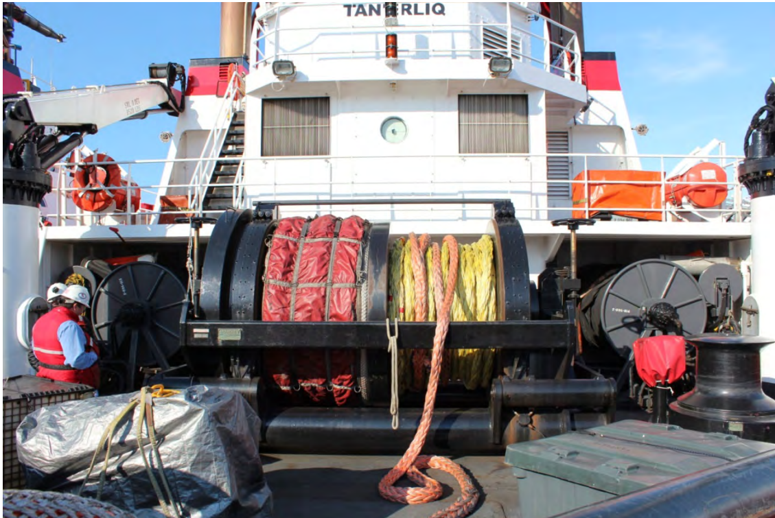
Figure D.13 - Main escort towing winch on the "aft" working deck of Tan'erliq . As with all tractor tugs, escort work is done over the aft end where the skeg is located, providing the lifting forces which help to generate high indirect steering forces.
