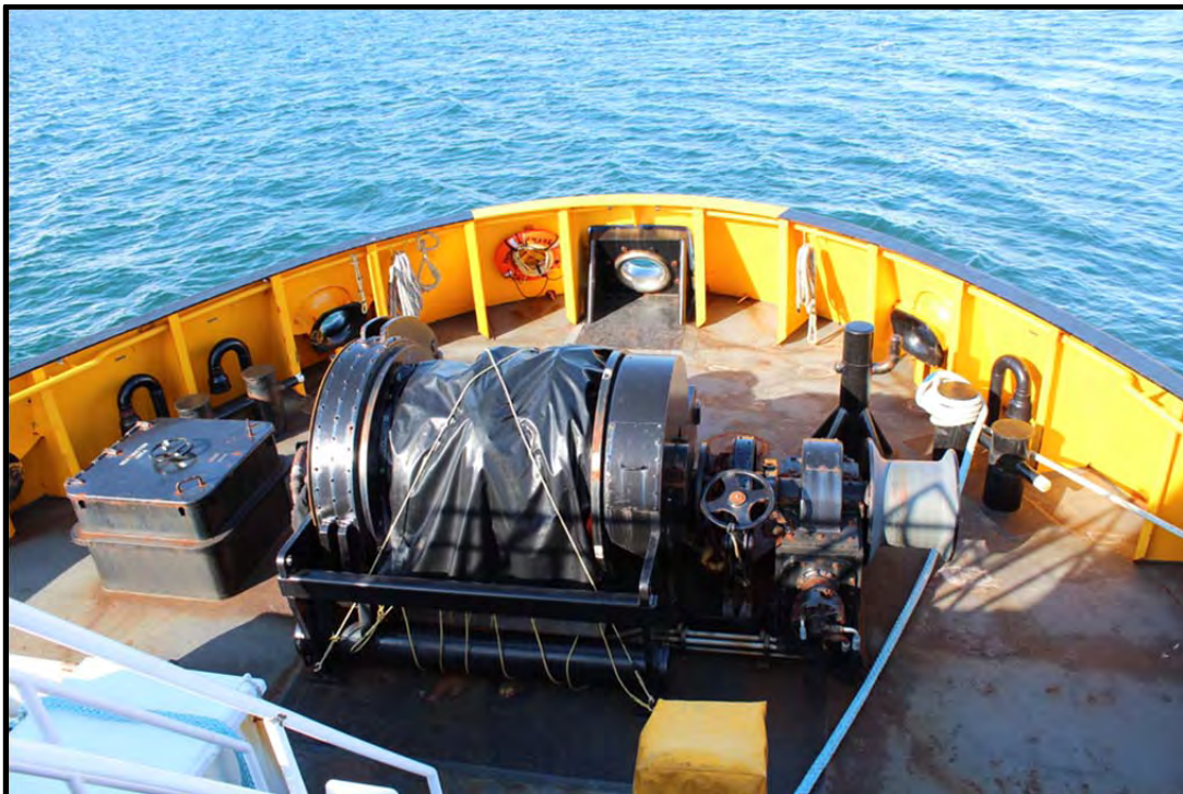
Figure D.8 - Fore deck layout showing winch and staple configuration.
