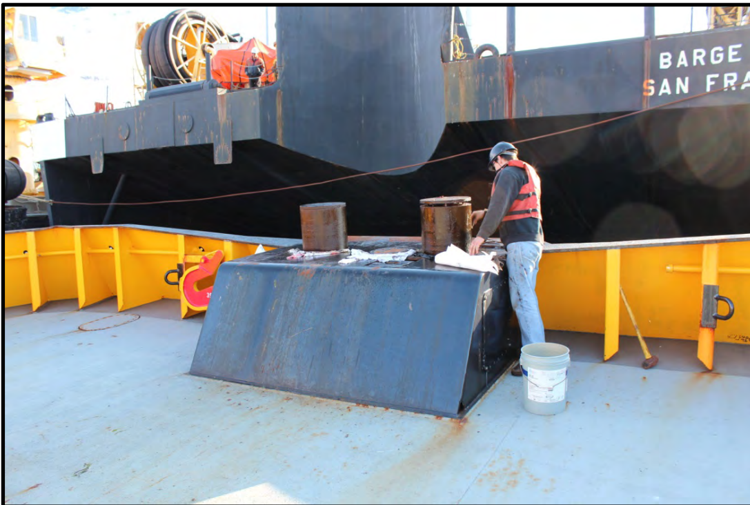
Figure D.5 - Retractable Stern Towing Pins at transom of Aware
