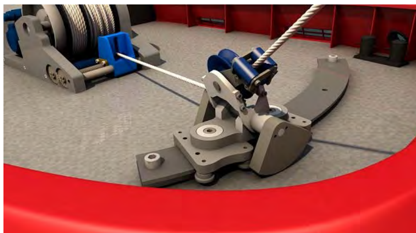
Figure 2.12 Kotug "Friction-Free Towing Device"
