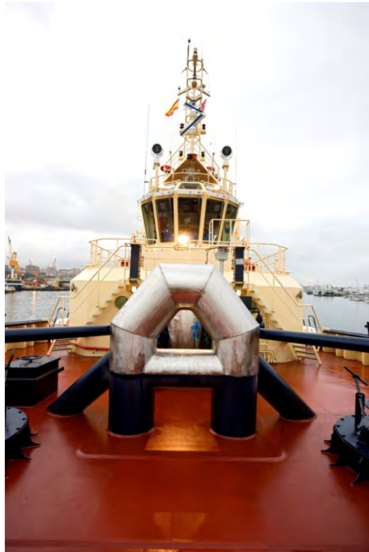
c. "A" Form Staple with Aft Bending Supports
