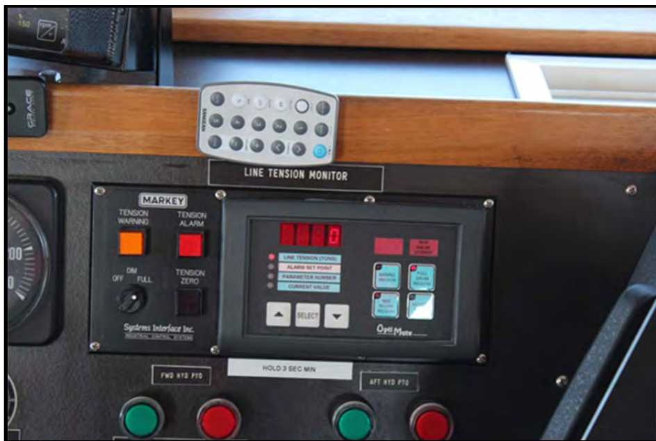
Figure D.12 - Line tension monitor on forward escort winch.
