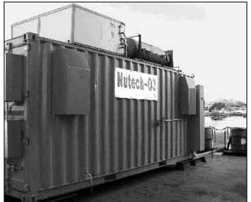
This module was installed on the Tonsina to generate ozone for the experiment in controlling non-indigenous species invasions. Photo by Rica Salvador.
