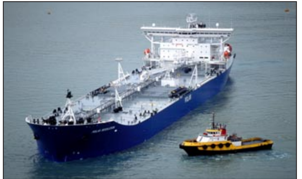
RESOLUTION — Phillips Petroleum's second new-build double-hulled tanker, the Polar Resolution , takes on its first load of North Slope crude at the Valdez Marine Terminal in July 2002. Phillips' first new double-hull, the Endeavour , started service a year earlier. The vessels will help Phillips comply with the Oil Pollution Act of 1990, which requires double-hull tankers to be phased in by 2015. Photo courtesy of Phillips Petroleum.
