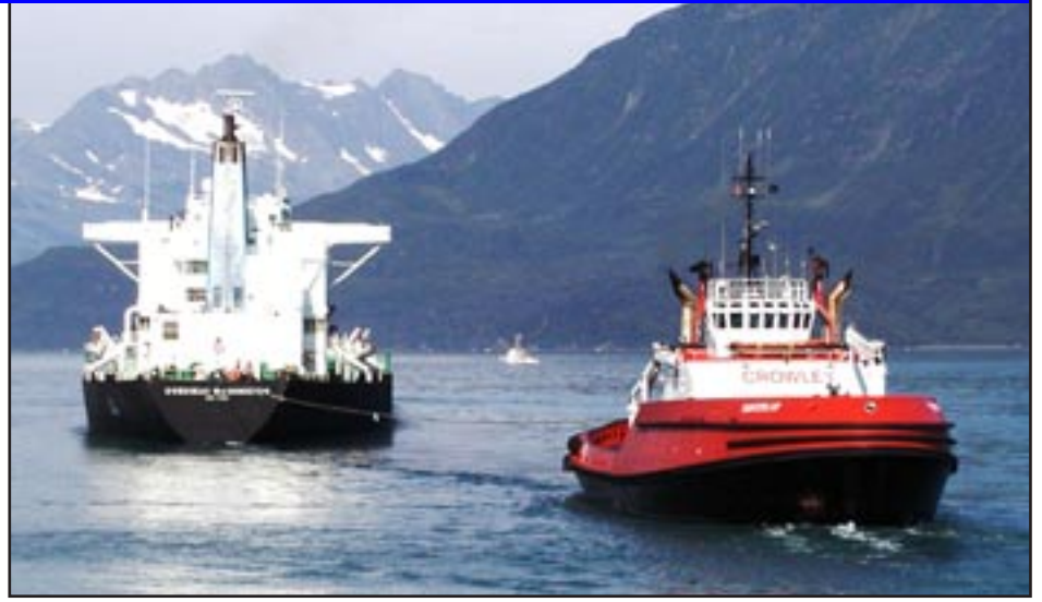
Above: The exercise begins with the two vessels in standard escort configuration for confined waters. The Tanerliq is tethered to the stern of the Washington , traveling backward as the tanker leaves port.
