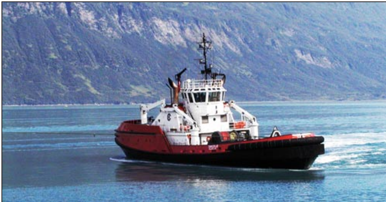
Left: Because of the force required to pull the tug sideways, it acts as a brake also, slowing the “crippled” tanker as it corrects the course.
