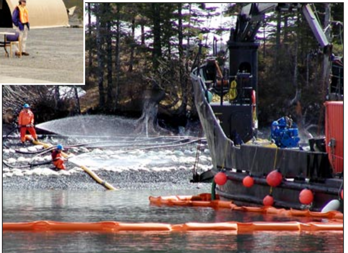
Above: BP set up a logistics base in Whittier to provide support for spill-response activities. Facilities included a warehouse area, shown here. Right: During the drill, but separately from it, Alyeska conducted a cold-water deluge exercise on this beach near Whittier. Water is pumped to the top of the beach. It flows downhill and washes oil into the white mops, or "pom-poms." Any oil that gets away is captured by the orange boom floating just off the beach.
