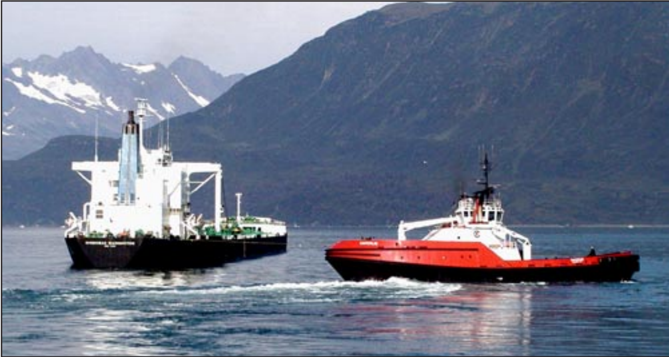
Left: Captain Steve Jones of the Washington starts the exercise by ordering the rudder hard over and stopping his engines. Captain Steve Walli of the Tanerliq swings the tug sideways to act as the tanker’s rudder, arresting the turn and then bringing the Washington back on course.
