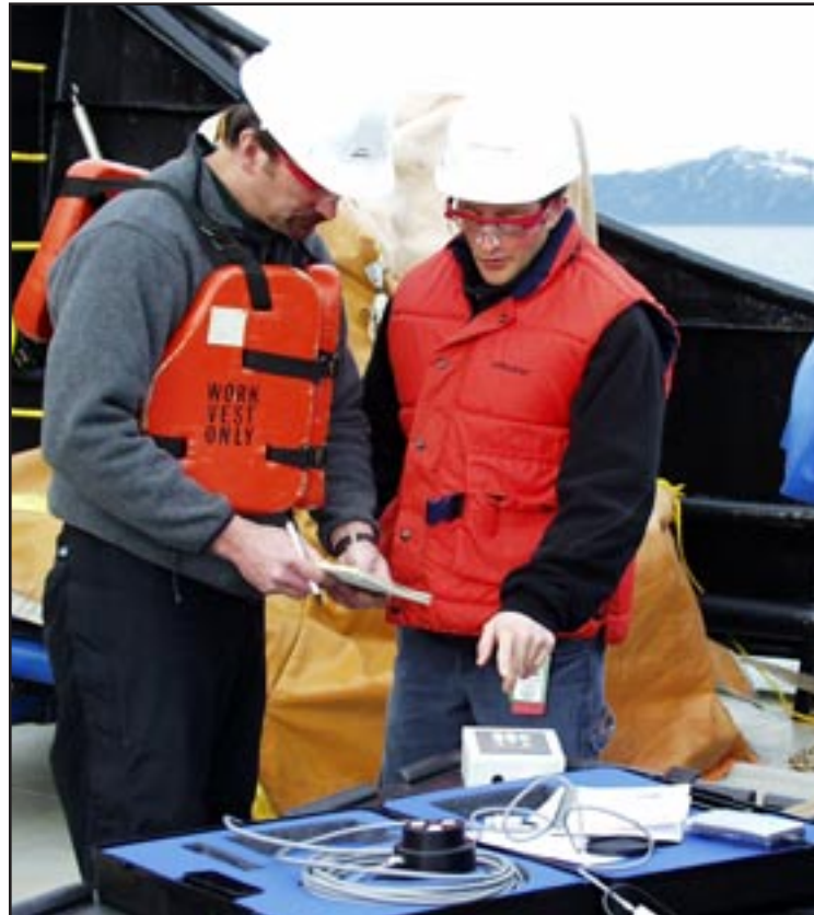
UV SAMPLES — Right, Dr. Mace Barron lowers a radiometer into the waters of Port Valdez as part of the council's ultraviolet light monitoring project. Above, Barron discusses use of the radiometer with council Project Manager Dan Gilson. Ultraviolet radiation is a component of sunlight that, while invisible to humans, increases the toxicity of oil. The purpose of the council's two-year project is to measure how much ultraviolet is present in subsurface waters of Prince William Sound. This information has not previously been available, but is critical to evaluating the risk and injuries from spilled oil and chemically dispersed oil in Prince William Sound. The project has just wrapped up its first season, in which 12 sites in Port Valdez and Prince William Sound were monitored. The work will
