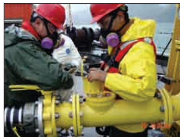
Participants in the Sept. 30 surprise drill check the flow rate from a TransRec oil skimmer. Flow rates are monitored so the tankerman can control the proper loading of the barge. The follow-up drill went better than the first surprise drill in June. Photo by John Engle, Alaska Department of Environmental Conservation.
