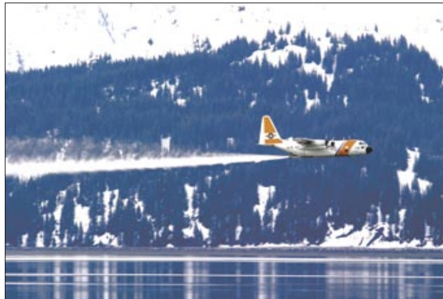
On April 19, the Coast Guard and Alyeska teamed up for a demonstration of how dispersants would be applied from aircraft if approved for use during an oil spill. Here, a Coast Guard C-130 makes a spraying pass over Port Valdez. For the exercise, water was substituted for dispersant. Photo by Pat Welch, Valdez.
