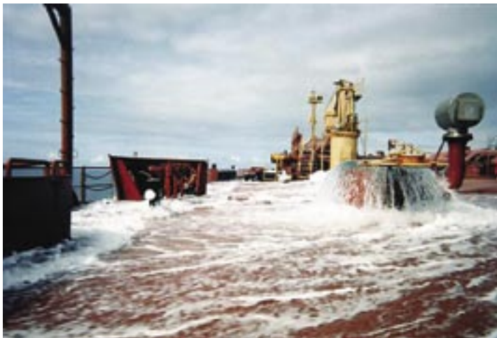
During exchanges, ballast water from port is discharged and replaced on the high seas. Here, ballast water is being pumped onto the deck and is running over the side. On other vessels, ballast water is discharged directly from the side of the ship. Photos courtesy of Smithsonian Environmental Research Center.
