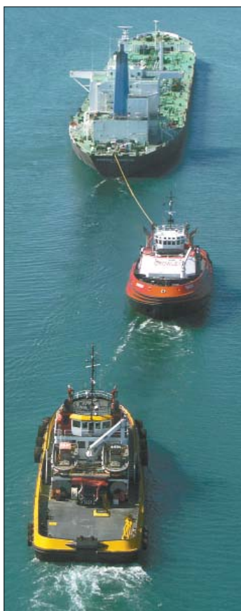
Current rules require two escort tugs for each loaded tanker. Photo courtesy of Alyeska Pipeline.
