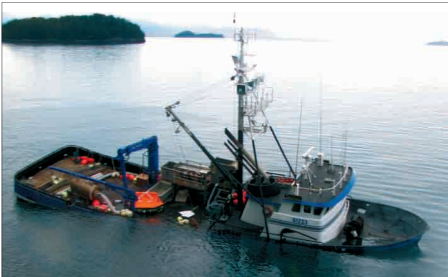
The Northern Mariner, a 91-ft vessel, intentionally grounded in shallow water on Flemming Island after the vessel struck a rock and experienced severe flooding. Photo courtesy of Alyeska SERVS.
