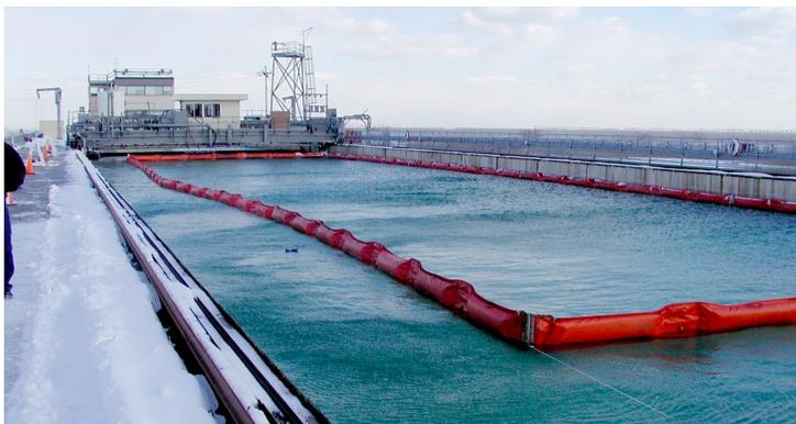
As part of this project, the council observes oil dispersant testing at Ohmsett, an oil spill research test facility in New Jersey. Ohmsett has a pool where oil and dispersants can be sprayed into the water without risk of contaminating the environment.
