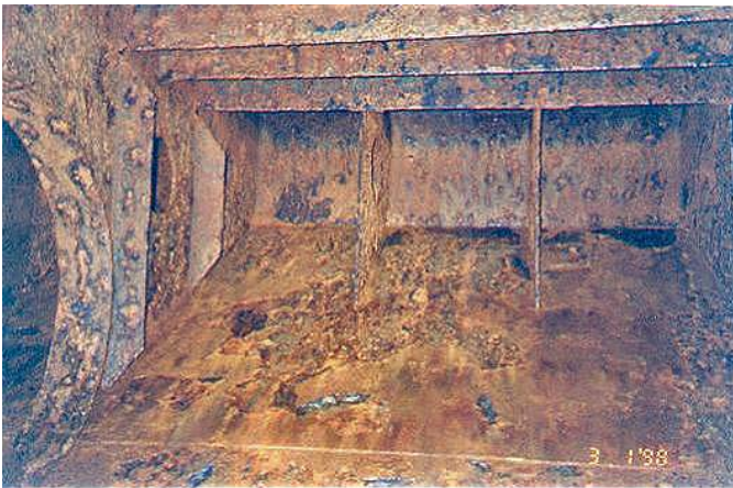
Figure 4.5 Improperly applied ballast coating leads to significant corrosion in another 13-year old vessel (Source: IACS)
