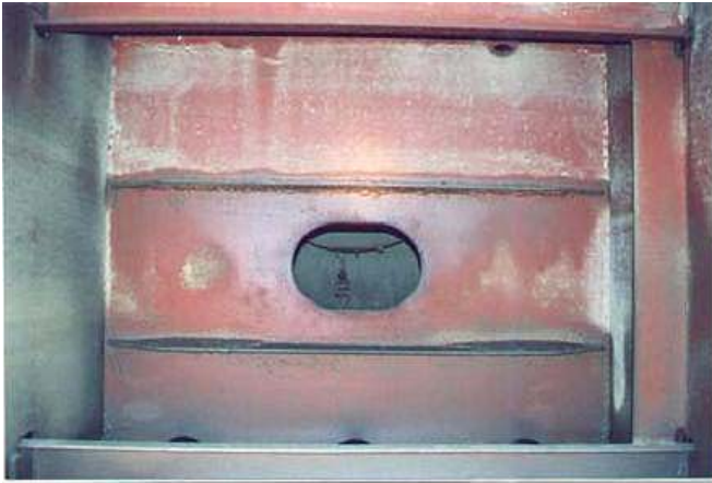
Figure 4.5 Improperly applied ballast coating leads to significant corrosion in another 13-year old vessel (Source: IACS)
