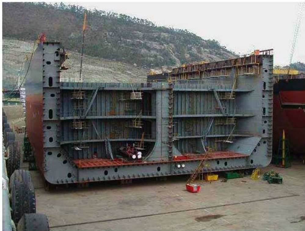
Figure 2.2 Double Hull Tanker under construction, showing tank spaces and double hull/ballast area (Source: AMSA, 2002)
