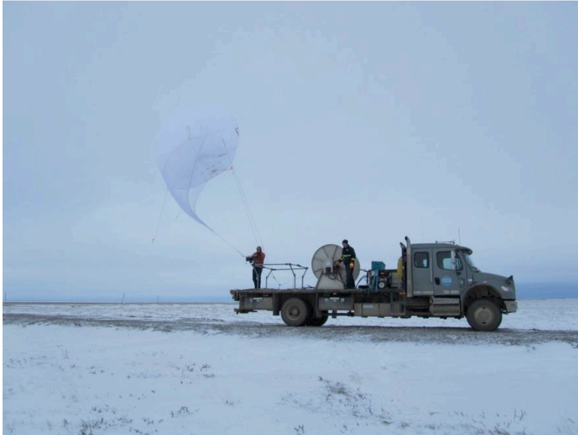
Figure 13. The balloon system was also tested by deploying it from a vehicle. Pictured are the balloon, camera being mounted, a docking station, and boom reel used as a winch. Photo courtesy of Alaska Clean Seas.
