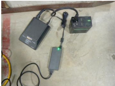
Figure 10. The battery connected to the battery charger.
