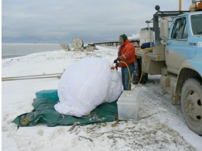
Figure 7. Beginning to fill the balloon. The yellow hose connects the fill nozzle (in hand) with the helium tanks on the truck.
