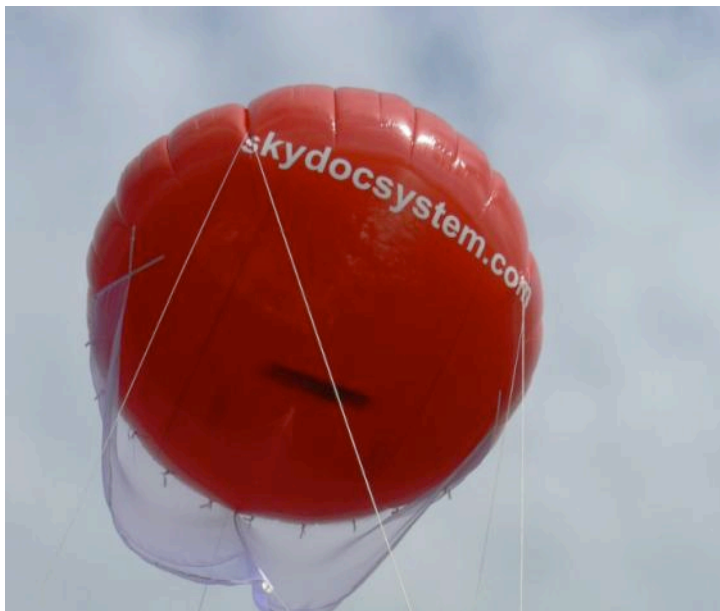
Figure 1. The red portion is the balloon that is filled with helium. It has a flattened shape and when there is wind the sail (white cloth below the balloon) orients the balloon into the wind. The balloon will also tilt backwards allowing the flatter bottom section to act as a kite with
