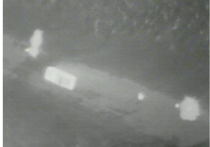
Figure 14. On left is a visible picture of a warm water spill, truck (second warm spill at the far right of picture), and person. On right is the same scene in IR. Cones at the location of the warm water can also be seen. The warm water goes under the snow yet remains visible because it can warm the snow up to freezing and the surrounding snow remains at air temperature.
