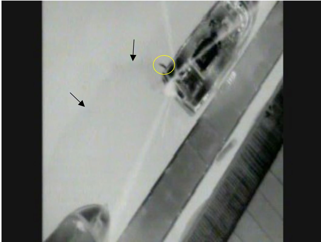
Figure 18. The cooling system plume from the generator is circled in yellow. It is ten degrees above the ambient temperature. The arrows point to the warmer water as it travels back. The temperature gradient is less than one degree between the two water masses. Under IR, PWSSC was able to watch this warmed exhaust water drift into the harbor and eventually, ten feet from the boat, cool back down and become indistinguishable from the surrounding water.
