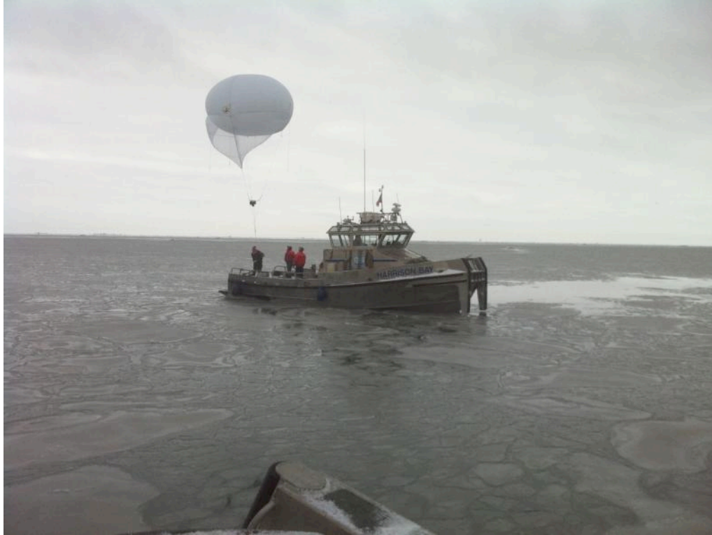
Figure 11. Pictured is the balloon system being deployed off the Alaska Clean Seas vessel Harrison Bay. A capstan was used to deploy and retrieve the balloon. During that test, no docking station was used, but rather the balloon was kept aloft at low altitude while underway. Photo courtesy of Alaska Clean Seas.
