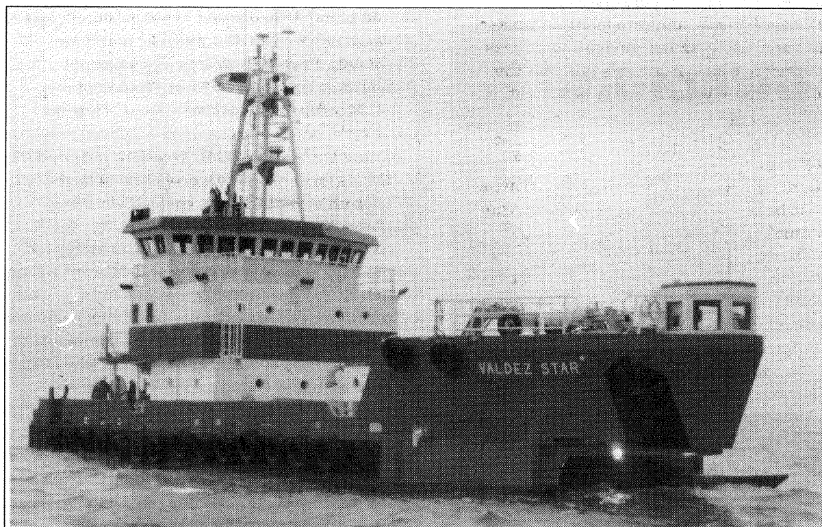
The "Alexandra" (above) was one of 12 fishing vessels that set boom in the skimmer exercise. Below, the "Valdez Star", a dynamic incline plane skimmer, is the centerpiece of spill response because of its effective skimming capabilities. Photos by Patti Saunders.
