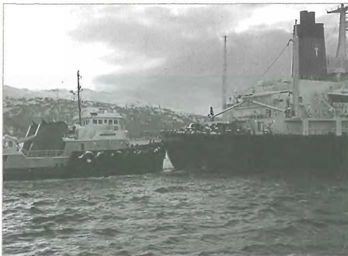
A tug is tethered to the tanker Overseas Boston. Close tethering ensures the tug can quickly assist the tanker if it experiences power or steering problems.
