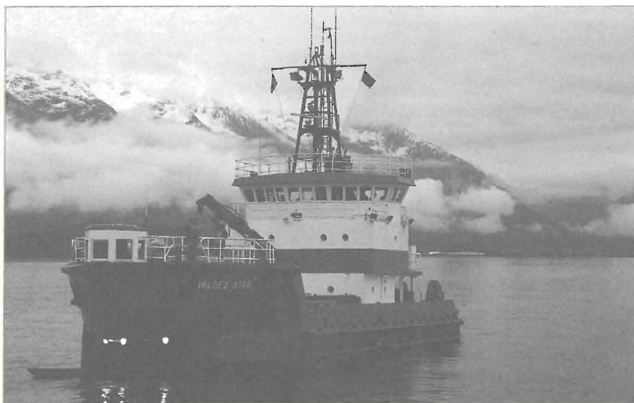
The Valdez Star, with its dynamic inclined plane skimming system, is an important component of Alyeska's Ship Escort/Response Vessel System (SERVS).
