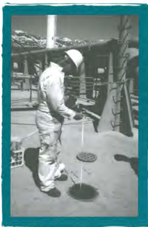
Tuck Hines, Smithsonian Environmental Research Center, measures the depth of the water in a segregated ballast tank prior to sampling for non-indigenous species in the ballast water. Photo by Joel Kopp.
