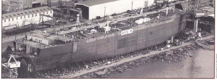
AN ARCO Millennium double-hull TANKER being ASSEMBLED in A LOUSIANA SHIPYARD for THE NORTH Slope oil TRADE.
