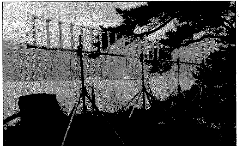
ICE WATCH -- This antenna was part of system set up on Busby Island last fall to test whether UHF radar can detect icebergs in the tanker lanes out of Valdez. Photo courtesy of C-CORE.
