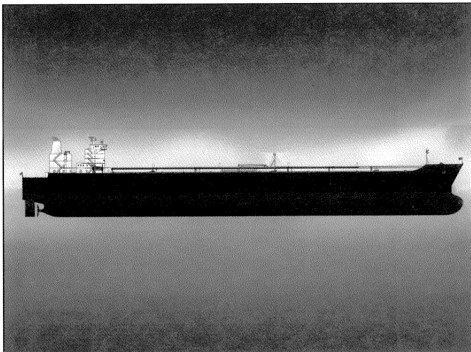
BP's Alaska Class Tankers will be 941 feet long and carry 1.3 million barrels of oil. The first is due in service in 2003. Illustration courtesy of BP
