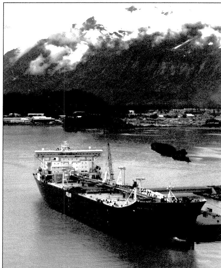
Phillips Petroleum's Polar Endeavour reached Valdez July 11. The Endeavour is the first double-hull tanker built for the North Slope oil trade under the Oil Pollution Act of 1990. Photo courtesy of Phillips Petroleum.
