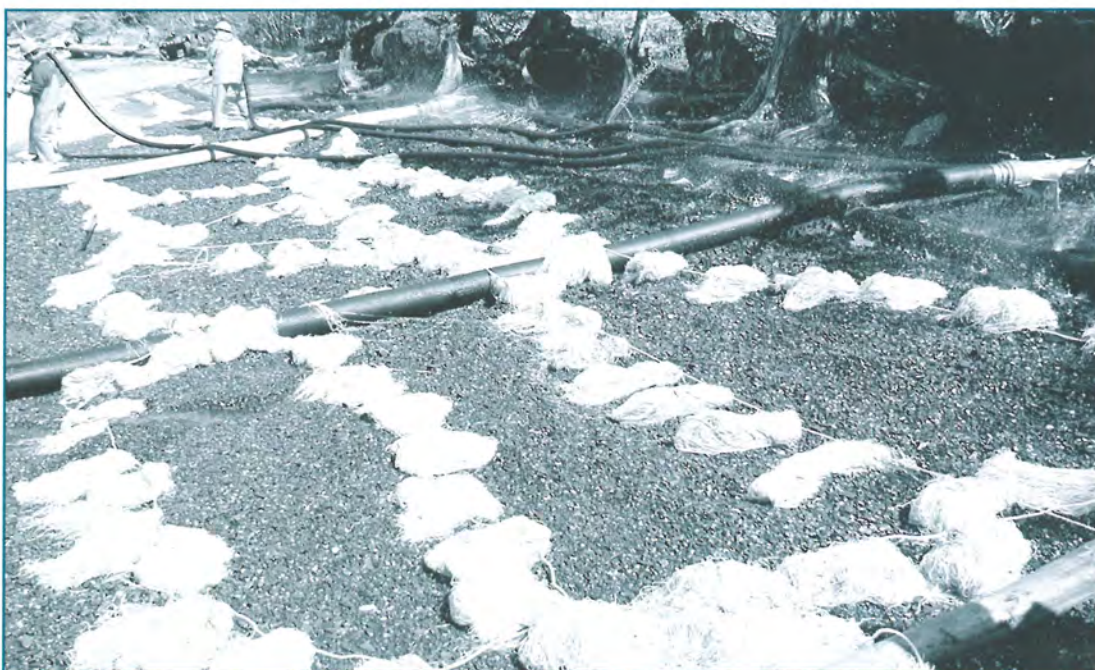
On the same day, Alyeska used this beach near Whittier to test a cleanup technique called cold-water deluge. Water is pumped to the top of the beach. It flows downhill and washes oil into the white mops, or "pom-poms."
