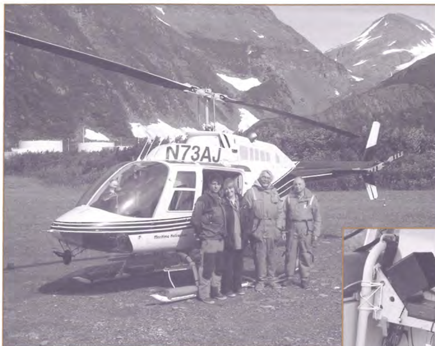
The ShoreZone mapping project uses a helicopter as an aerial camera platform to photograph shorelines (left). The system (below) includes a video camera and a computer for storing data.
