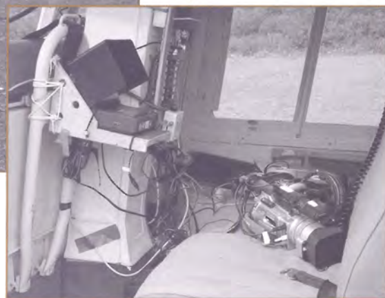
The ShoreZone mapping project uses a helicopter as an aerial camera platform to photograph shorelines (left). The system (below) includes a video camera and a computer for storing data.
