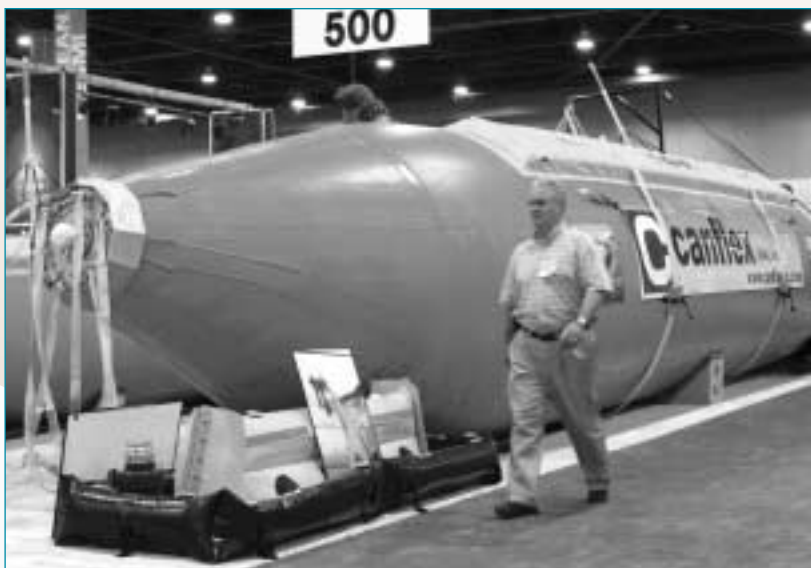
The Sea Slug, a giant bladder for holding recovered oil in a spill, was on display at the International Oil Spill Conference in Miami Beach in May 2005.
