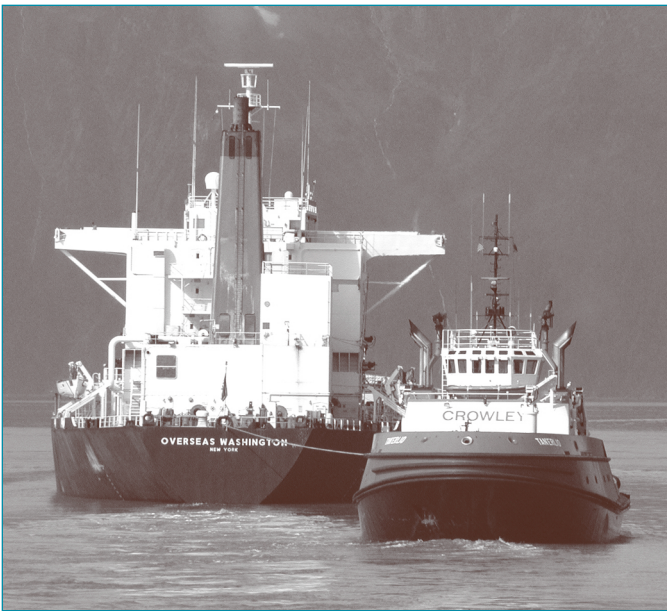
Loaded oil tankers in Prince William Sound are escorted by two powerful tugs. For part of the trip, one must be tethered to the tanker's stern for immediate response in emergencies.
