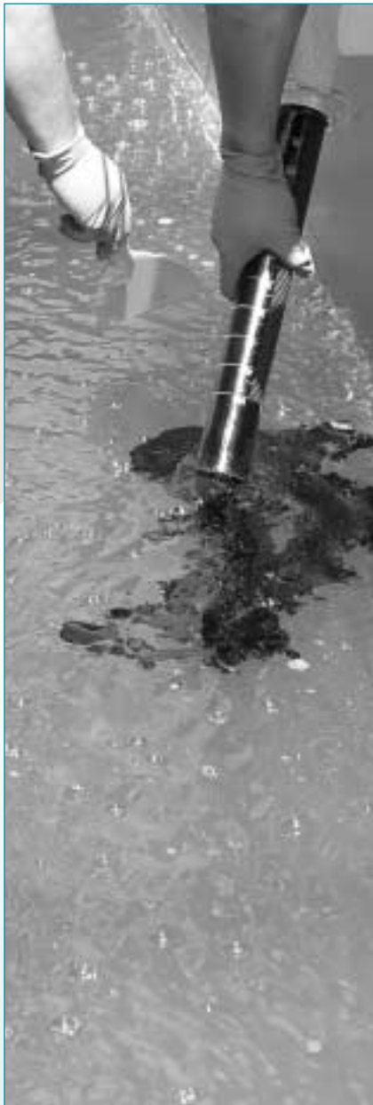
Oil is poured into a Canadian seawater tank designed to test chemical dispersants.
