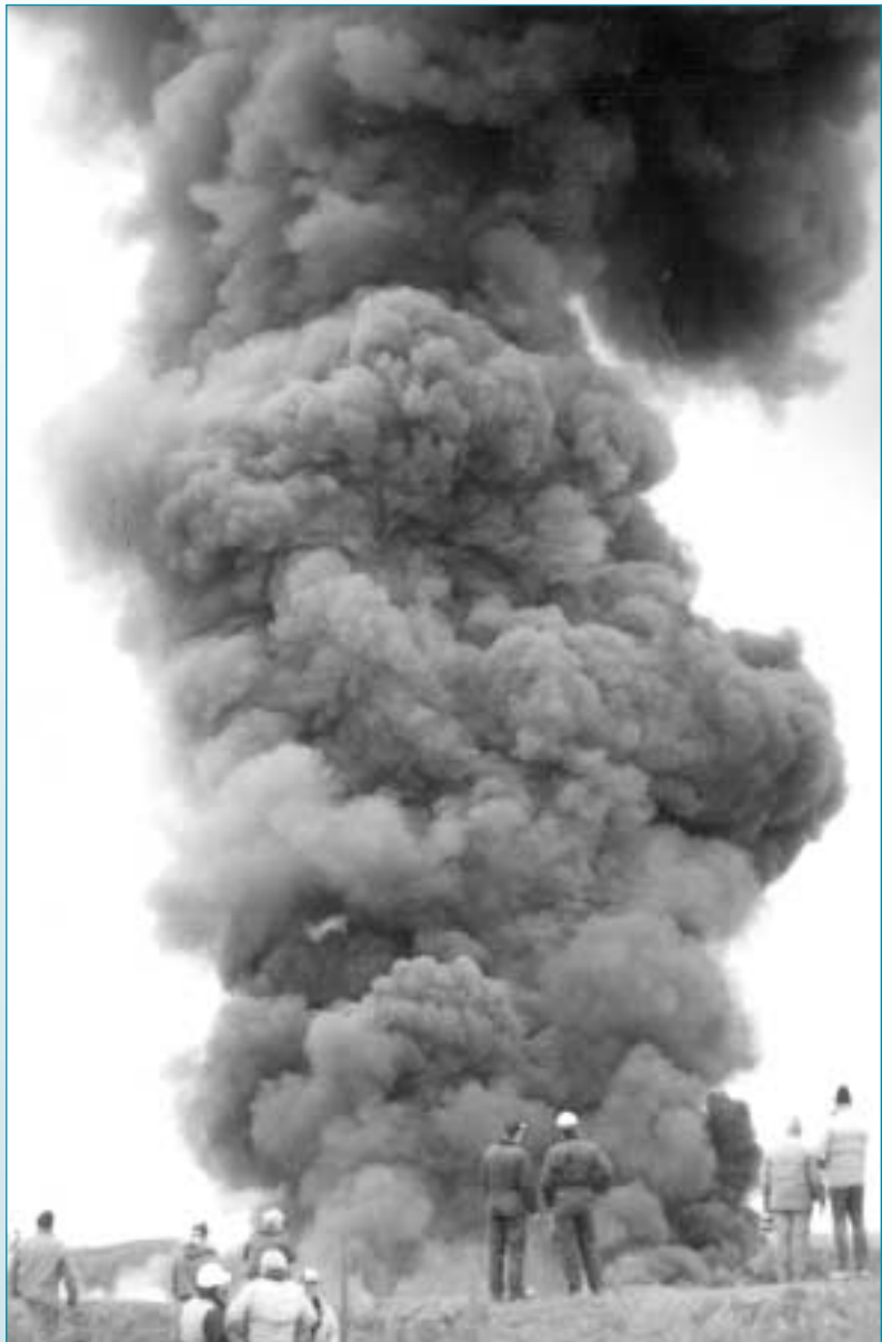
In-situ burning refers to burning oil where it spills. This photo shows an in-situ burning test on the North Slope in 1994.
