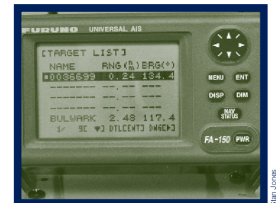
The council operates a Furuno Automatic Identification System in its Valdez office. The device shown here is part of a system that archives traffic information, as well as feeding it to a large video screen in the office.
