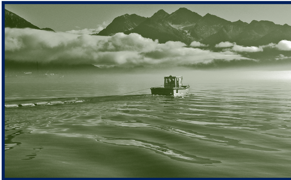
Though the council opposes the use of dispersants on oil spills, they remain on the list of approved response tactics, and Alyeska crews practice dispersant application from time to time. Here, one of Alyeska's escort tugs uses a dispersant spraying apparatus during an exercise near Valdez.
