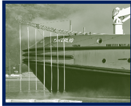
Though the council opposes the use of dispersants on oil spills, they remain on the list of approved response tactics, and Alyeska crews practice dispersant application from time to time. Here, one of Alyeska's escort tugs uses a dispersant spraying apparatus during an exercise near Valdez.
