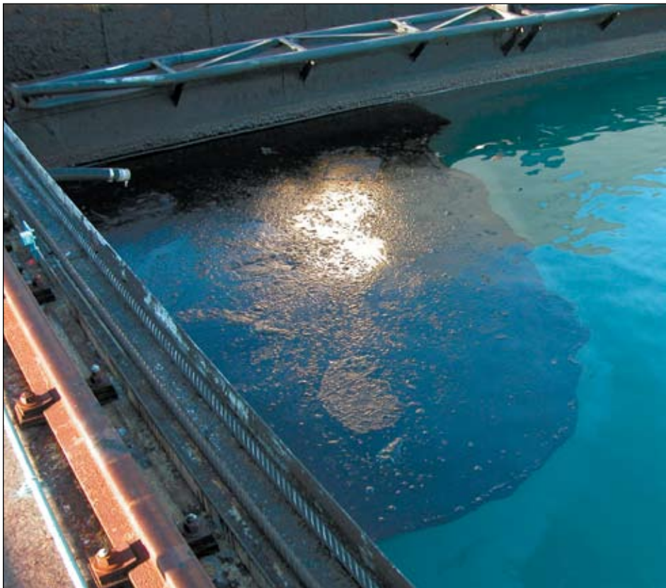
Resurfaced oil, shown here in a corner of the OHMSETT test tank, is a serious, persistent, problem observed by the citizens' council in several years of monitoring dispersant demonstrations at the facility. Photo courtesy of Merv Fingas.
