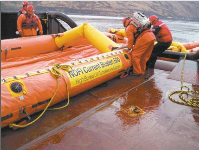
A CurrentBuster skimming system aboard the Endurance is inflated for deployment.
