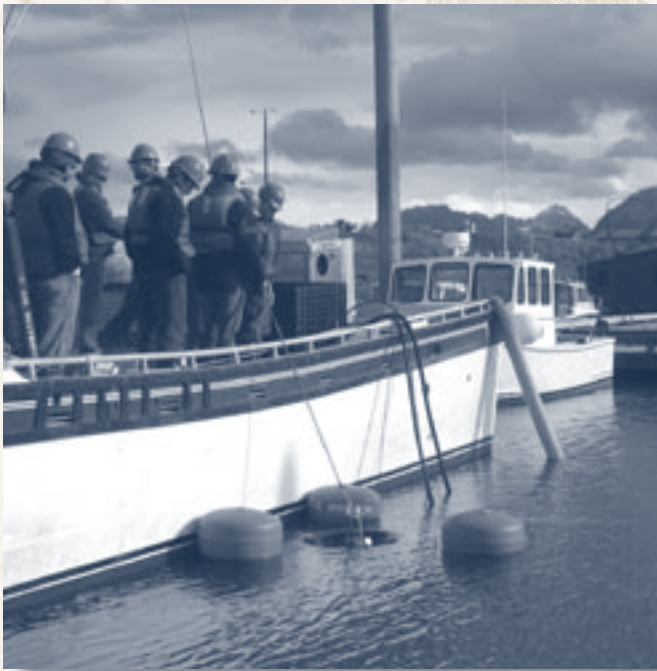
A fishing vessel participates in a training exercise near Homer in October 2006. The equipment alongside is part of a system for skimming floating oil off the water. Photo by Susan Sommer.
