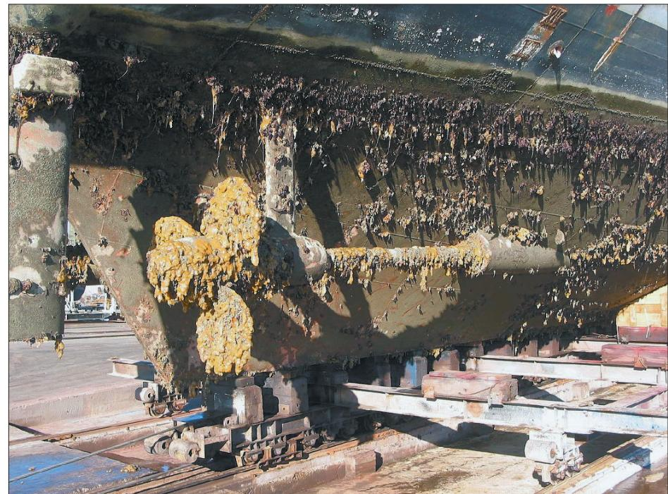
**HITCHHIKERS**—When this ship entered dry dock in New Zealand, its hull, propeller shaft, and propeller were heavily encrusted with biofouling organisms. Photograph by Tim Dodgshun, Cawthron Institute, Nelson, New Zealand.
