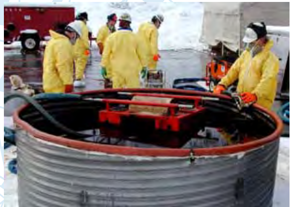
Contractors with Alyeska Pipeline receive training in use of an oil skimmer. The tank contains water with a layer of real oil on top. Photo by Dan Gilson.
