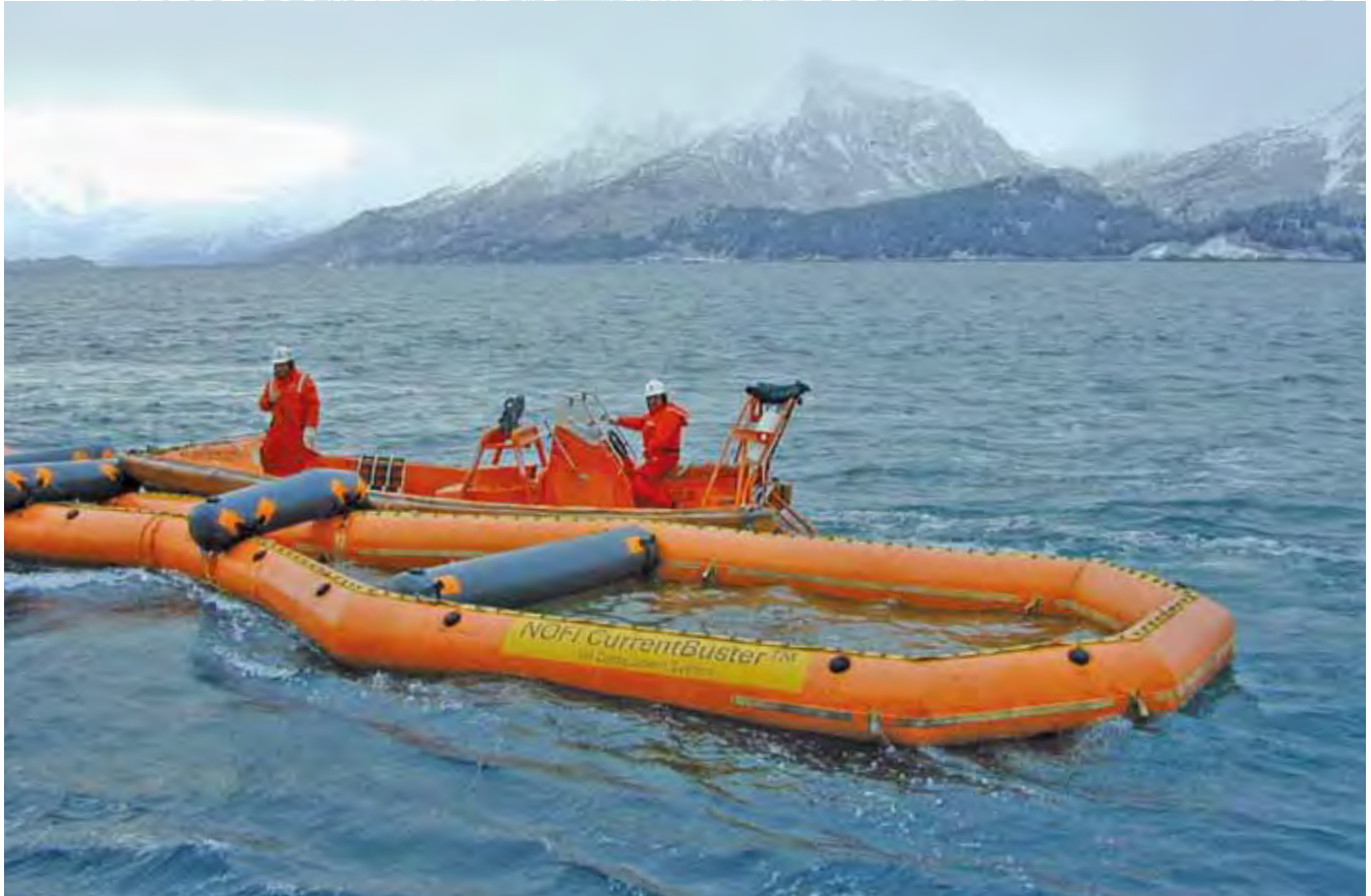
These men are deploying a high-performance oil booming and skimming system called the CurrentBuster. Photo by Becky Lewis.
