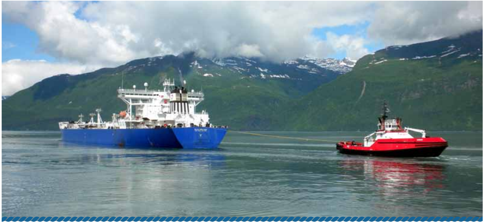
→ The escort tug Nanuq is tethered to the stern of the tanker Polar Endeavor as it travels out of Prince William Sound with a load of oil. This photo was taken from the tanker's other escort tug. Photo by Tom Kuckertz.
