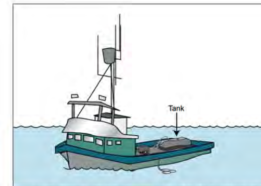
Figure 5. Generic tender vessel with deck-loaded storage tank for offloading oil collected by CRDF Tender-based Nearshore Free Oil Recovery Strike Teams (STAR Manual)
