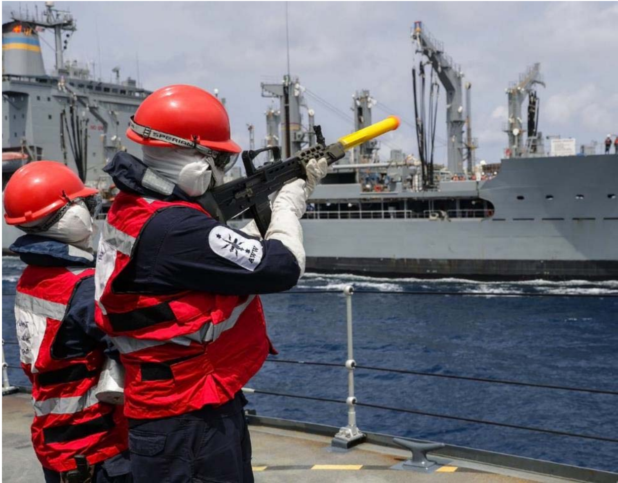
Figure 5 Photo of a British Royal Navy Warfare Specialist officer preparing to fire a soft nose projectile from an adapted SA80 shoulder line throwing gun; photo from twitter.com/navylookout
