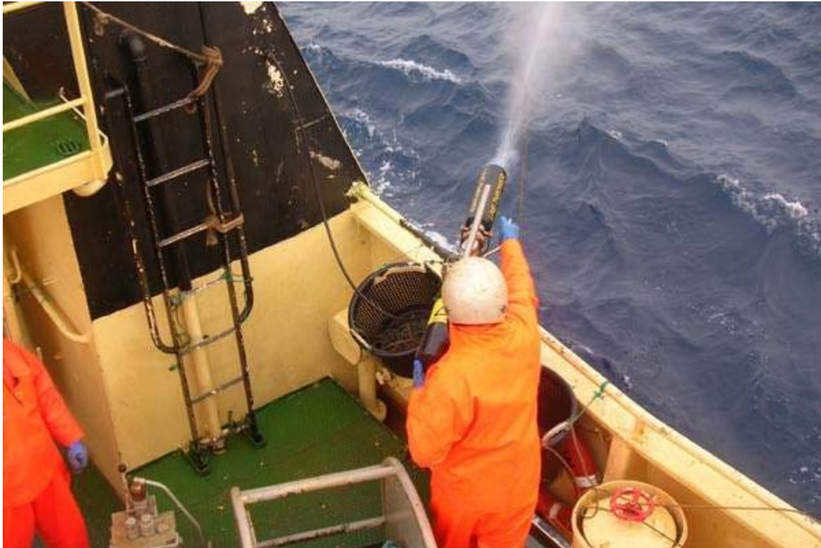
Figure 4 Photo of a pneumatic type line-throwing device (Vonin L-75) being activated from the deck of a vessel at sea; photo from ship-technology.com
