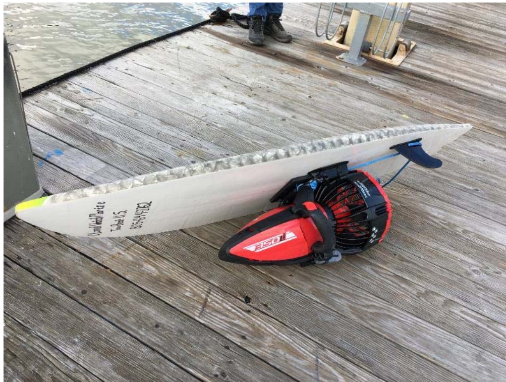
Figure 8 Photo of a prototype waterborne drone for delivering a messenger or towline to stranded/grounded vessels; this unit is constructed of a Yamaha 350Li Seascooter mounted to the bottom of a molded high-density polyethylene surfboard
