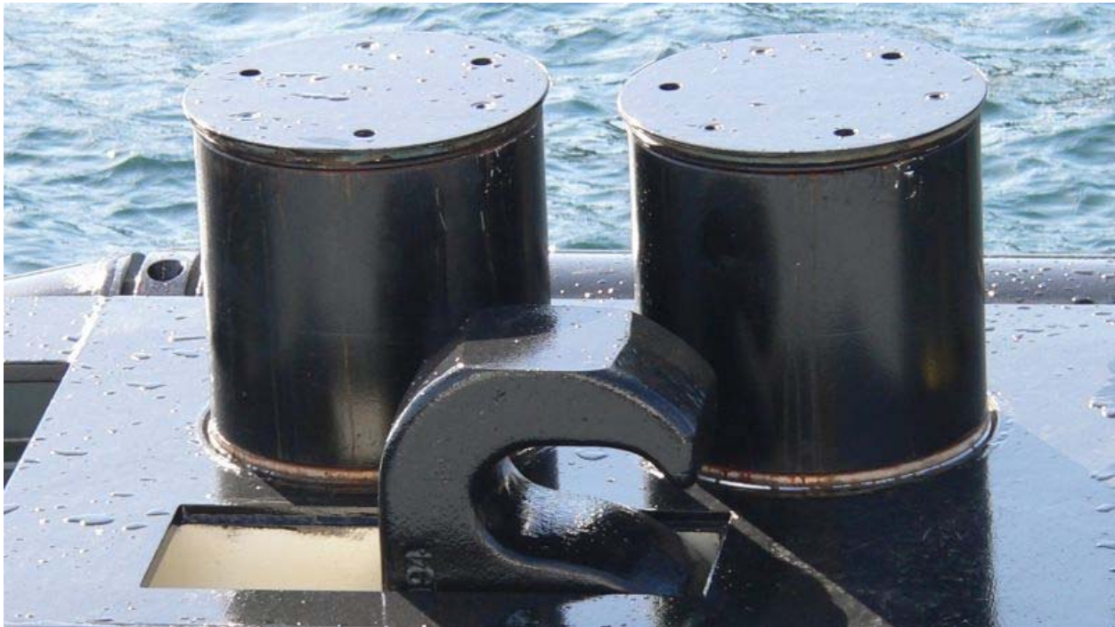
Figure 4 Photo of the conventional Smith Berger tow pin and hook assembly installed on the current SERVUS escort tugs, accessed from https://maritime-executive.com/corporate/tow-pins on 3/20/2021
