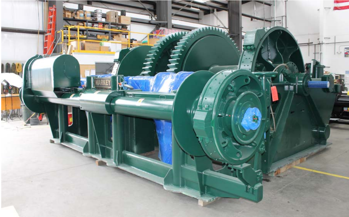
Figure 2 Example of a side-by-side double drum ocean towing winch, configured for underwound wire deployment; photo courtesy of Markey Machinery
