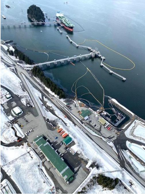
Fig. A4-2. Containment booms placed around the spill site and in adjacent waters. Saw Island in upper left background. Image from Alyeska Pipeline.
