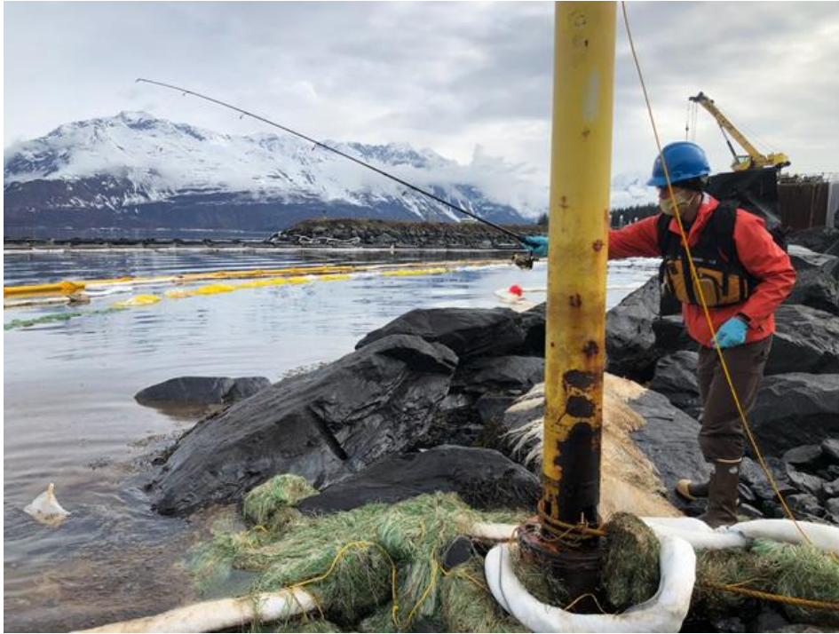
Fig. A4-3. Austin Love collecting the intertidal source-oil sample with a Teflon® net on April 30, 2020.
