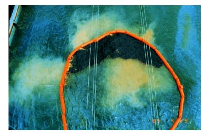
Figure 8 A dispersant test underway at the Imperial test tank in Calgary, Alberta. This tank has since been demolished.
