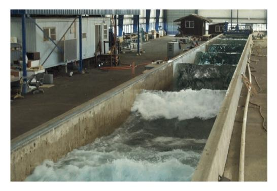
Figure 16 Oregon State large wave flume. This tank may be a candidate for dispersant testing.
