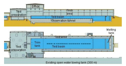
Figure 29 Schematic of the Hamburg large tank for ice testing
