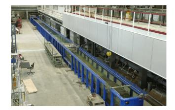
Figure 26 A glass-lined flume at Delft
