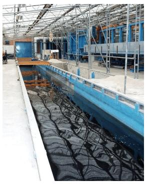
Figure 38 Environmental tank at VWS in Berlin. This tank is used to test behaviour and cleanup of oil and other hazardous materials.
