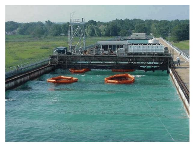
Figure 5 Testing in circular booms being conducted at the OHMSETT tank. The towed bridge is used to discharge oil and take samples.
