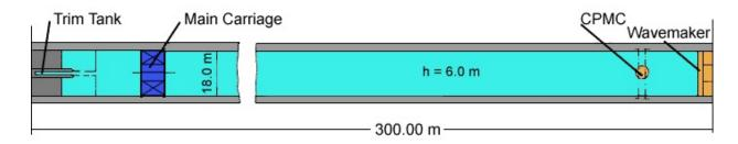
Figure 27 Schematic of the large tow tank at the Hamburg Shipbuilding Facility
