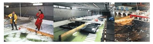
Figure 28 Montage of photographs of the Hamburg ice tank. The photo at right shows an oil skimmer being tested.
