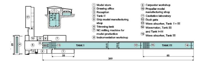
Figure 31 Tandem tow tank schematics at SINTEF in Norway
