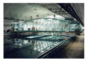
Figure 33 The tow tank at the National Marine Institute in Japan. This tank has the largest water volume of its type.
