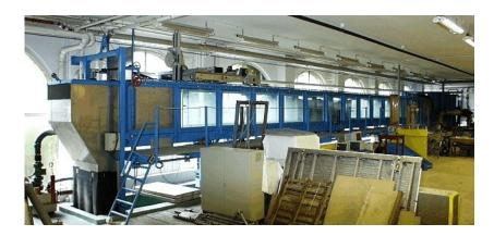
Figure 37 Tilting oil flume at VWS in Berlin
