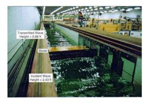
Figure 22 A wave at the National Research Council test tank in Ottawa, Ontario
