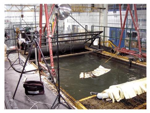
Figure 9 A skimmer being tested at Environment Canada's test tank.
