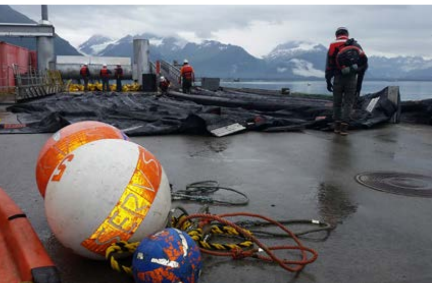
Boom is staged on an oil spill response barge during an exercise to protect coastline. Photo credit: PWSRCAC/Jeremy Robida.
