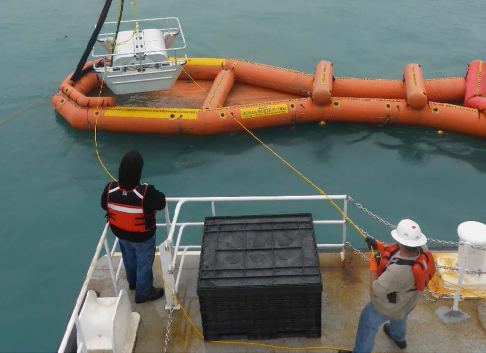
Crew trains with boom and crucial skimmer during 2018 oil spill response training. Photo credit: PWSRCAC/Jeremy Robida.
