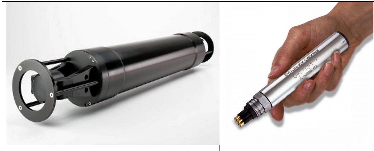
FIGURE A1. SEQUOIA LISST PARTICLE SIZE ANALYZER (LEFT) AND TURNER CYCLOPS-7 FLUOROMETER, WHICH CAN BE INTEGRATED WITH THE SEQUOIA TO MEASURE OIL CONCENTRATIONS BELOW A DISPERSED OIL SLICK TO ESTIMATE EFFECTIVENESS AS PART OF TIER 2 MONITORING
