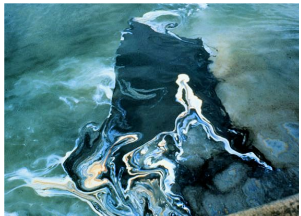
Dispersant was applied to this heavy oil slick but the dispersant ran off the slick without effective dispersion.
