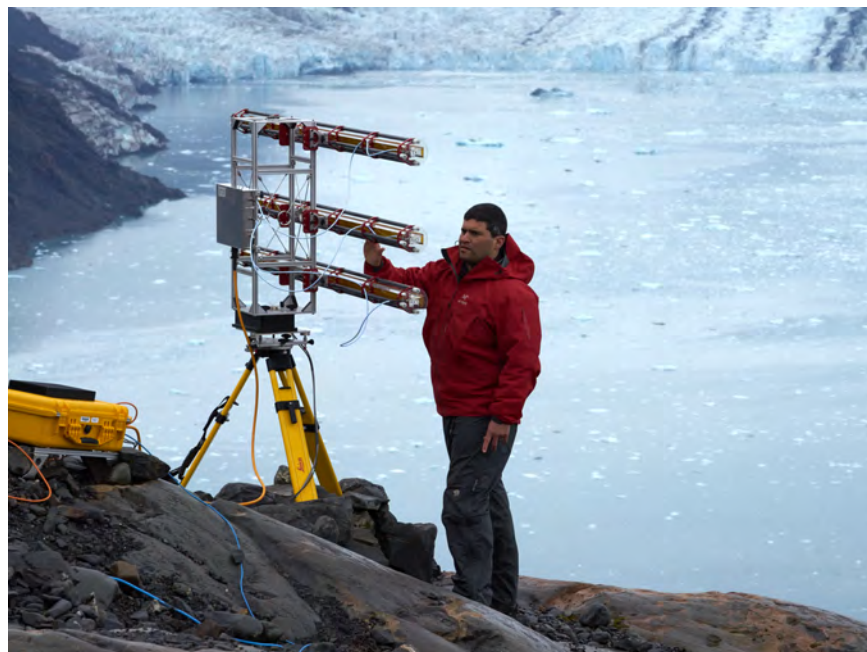
Figure 4. Gamma Remote Sensing Portable (GRSP) Radar Interferometer as installed at Columbia Glacier terminus.
