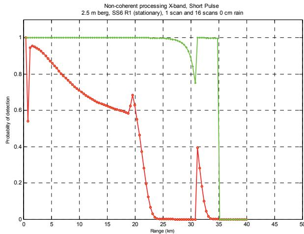
Figure 9. Iceberg POD versus range for Reef Island Radar for a 2.5 m iceberg for sea state 6. The plot compares scan averaging (green) versus no scan averaging (red).
