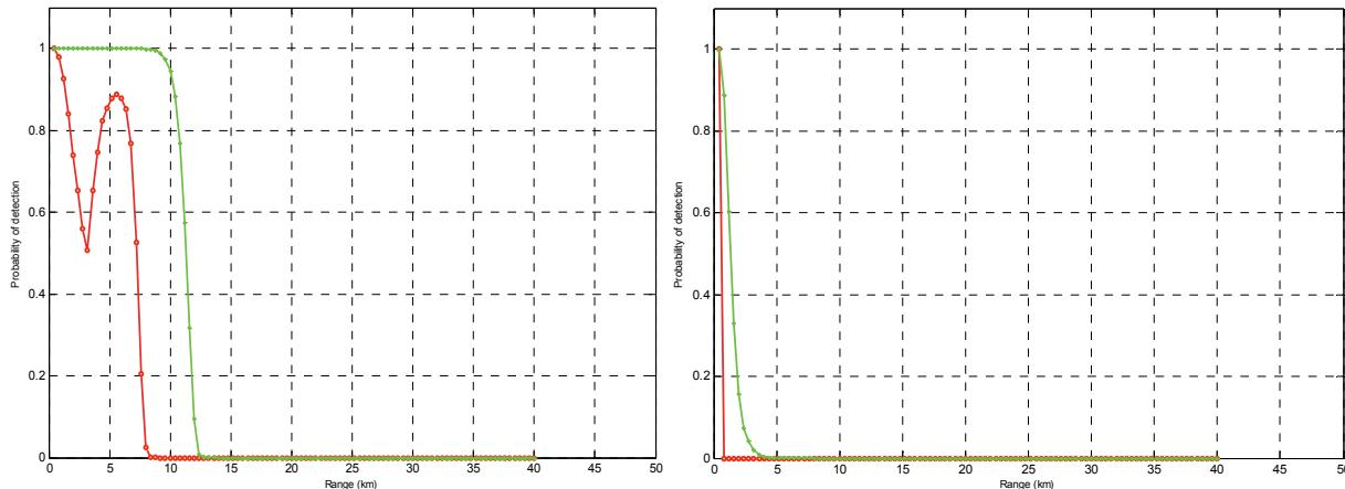
Figure 6. Iceberg POD versus range for the pilot vessel radar for a 2.5 m iceberg for sea state 4 (left) and sea state 6 (right). The plot compares scan averaging (green) versus no scan averaging (red).
