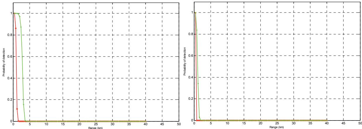
Figure 8. Iceberg POD versus range for the pilot vessel radar for a 2.5 m iceberg for sea state 4 (left) and sea state 6 (right) and 5mm/hr rain. The plot compares scan averaging (green) versus no scan averaging (red).
