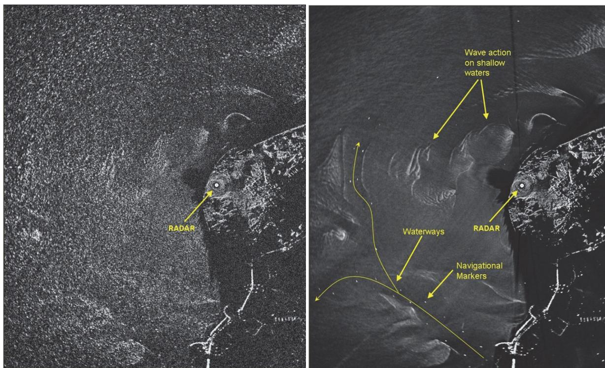
Figure 2. Example of Sigma S6 processing – (left) normal radar return, (right) reduced clutter through scan-to-scan processor (images supplied by Rutter Inc.)
