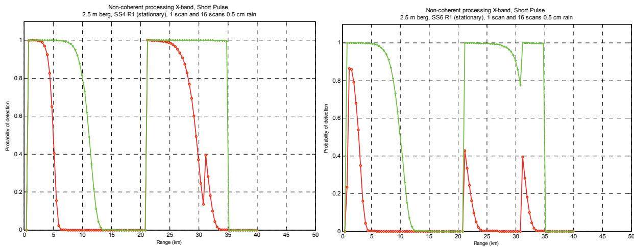
Figure 10. Iceberg POD versus range for the Reef Island Radar for a 2.5 m iceberg for sea state 4 (left) and sea state 6 (right) and 5mm/hr rain. The plot compares scan averaging (green) versus no scan averaging (red).
