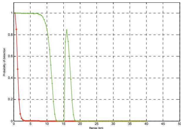
Figure 7. Iceberg POD versus range for the pilot vessel radar for a 5 m iceberg for sea state 6. The plot compares scan averaging (green) versus no scan averaging (red).
