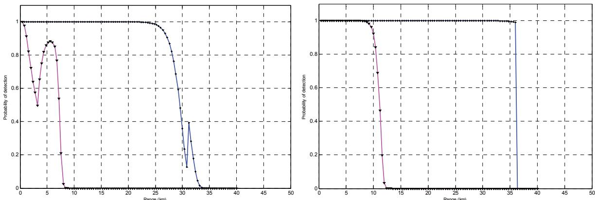
Figure 3. Iceberg POD versus range for Reef Island (blue line) versus pilot vessel (red line/ triangle markers) for a 5 m iceberg (right) and a 2.5 m iceberg (left) at sea state 4.
