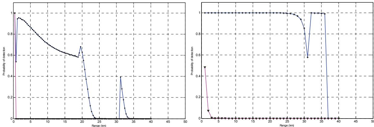
Figure 4. Iceberg POD versus range for Reef Island (blue line) versus pilot vessel (red line/ triangle markers) for a 5 m iceberg (right) and a 2.5 m iceberg (left) at sea state 6.
