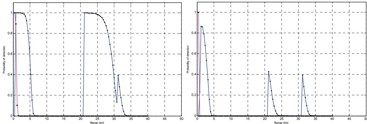
Figure 5. Iceberg POD versus range for Reef Island (blue line) versus pilot vessel (red line/ triangle markers) for a 2.5 m iceberg for moderate rain (5mm/hr) for sea state 4 (right) and 6 (left).
