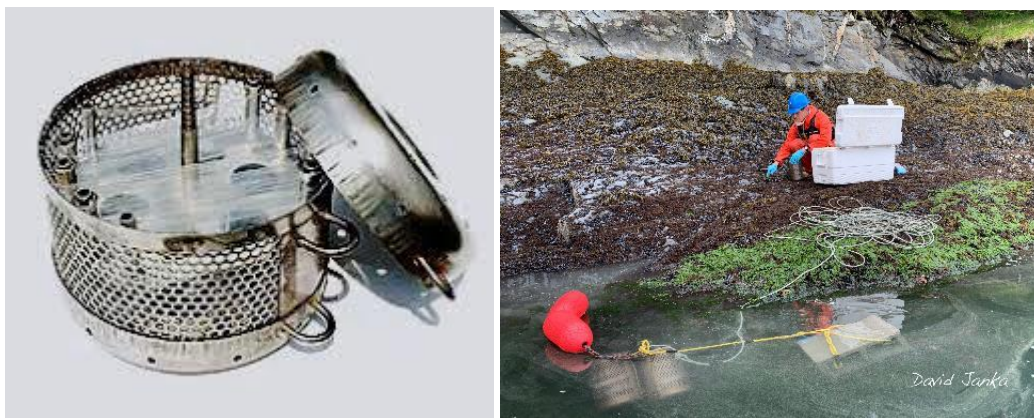
Figure 24. Passive sampling devices (PSD) consisting of a low-density polyethylene membrane enclosed in a stainless-steel container and deployed subsurface in near-shore subtidal waters adjacent to LTEMP mussel collection sites for up to 30 days prior to mussel sampling. Sampling photo courtesy of David Janka.
