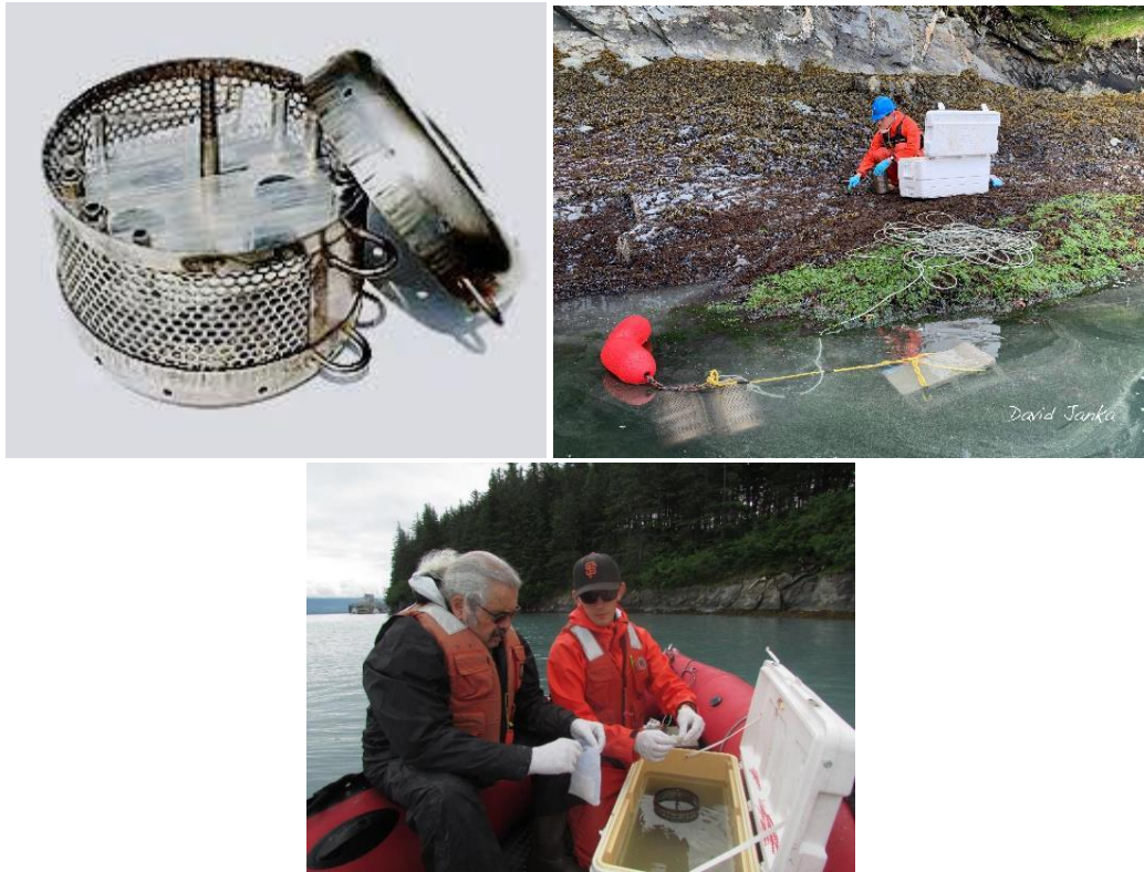
Figure 32. Example of passive sampling device (PSD) consisting of a low-density polyethylene membrane strip enclosed in a stainless-steel container and deployed subsurface in near-shore subtidal waters adjacent to LTEMP mussel collection sites. Work photos courtesy of David Janka.
