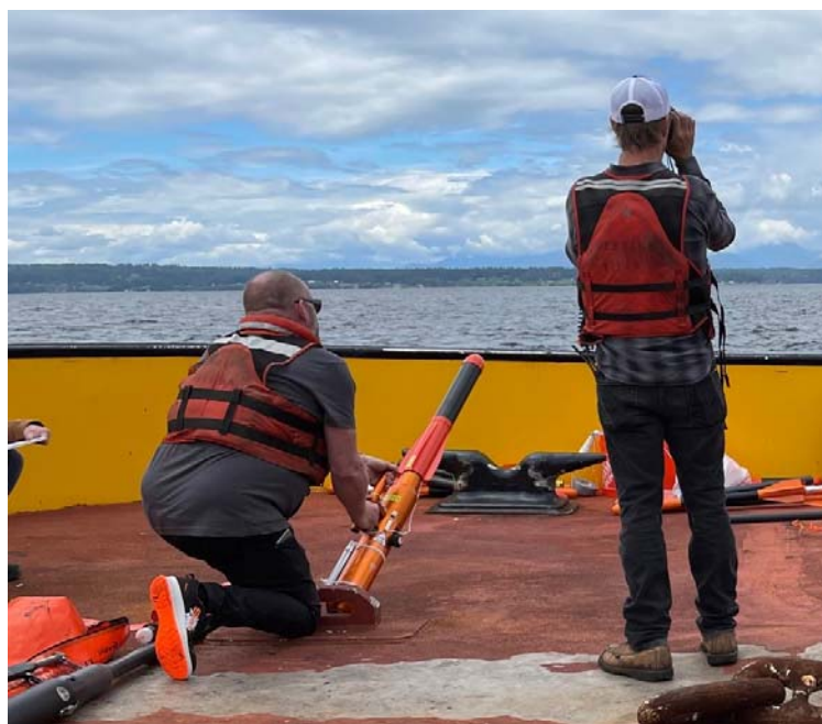
Figure 1 PLT-SOLAS being fired from padeye installed on the ETV aft deck
