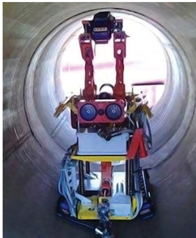
Robotic crawlers such as this one are now used to examine the interior of the pipes.
