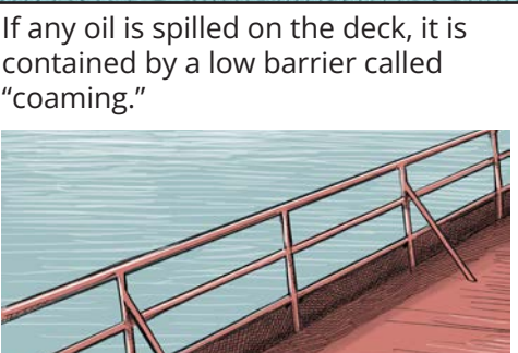
If any oil is spilled on the deck, it is contained by a low barrier called "coaming."
