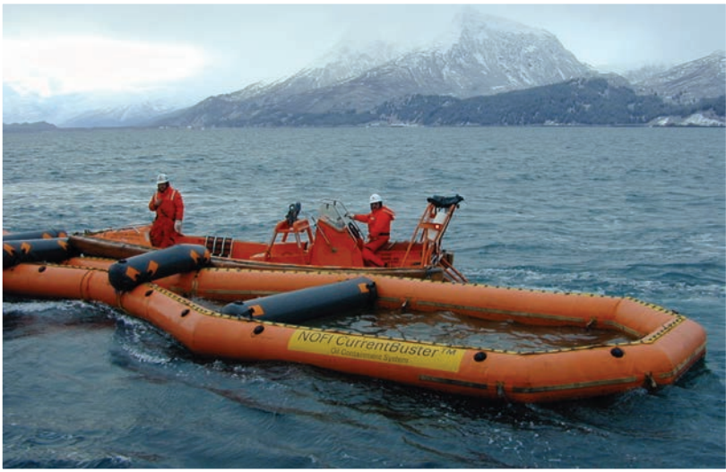
A council study is released in October 2008 that shows that Alyeska’s Current Buster skimming system, adopted three years earlier, can collect spilled oil up to five times better than the traditional “U” configuration
