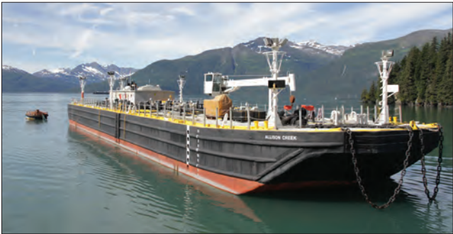
Storage tank barges such as the Allison Creek, pictured here during the August 29 spill response exercise, are used to store the oil and water mix recovered after an oil spill. Photo by Jeremy Robida.
