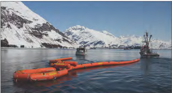
Left: Crews spend one day on the water practicing response techniques. Here, two fishing vessels practice pulling a "buster" oil spill boom system during the Valdez training. SERVVS' spill response tool-box contains differ-
