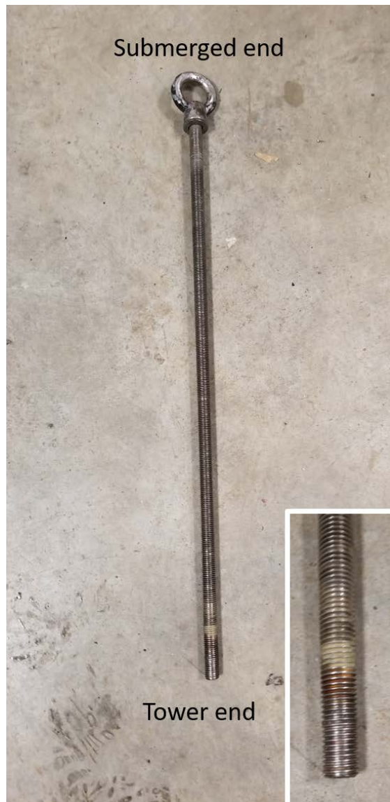
Figure 8: The threaded rod to which the remaining mount was attached. Inset: a close-up of the section that was threaded into the tower mount. No major corrosion is evident.
