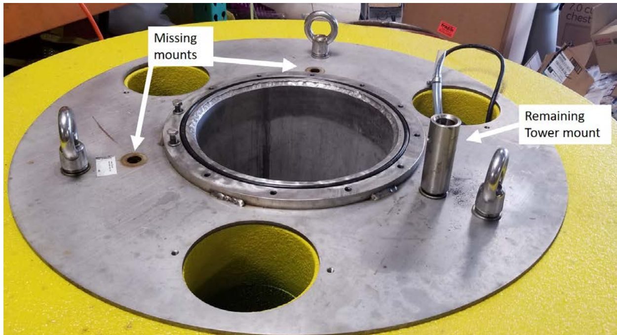
Figure 7: The top of the buoy hull post-failure.
