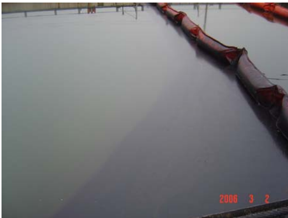
Resurfaced oil the morning after Test 6
