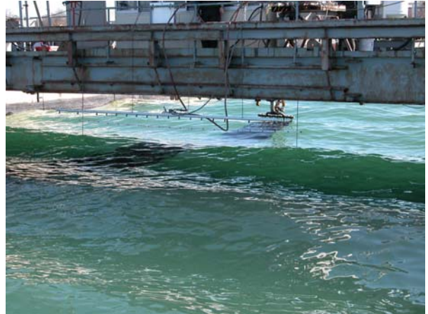
Oil nozzle and dispersant boom mounted on bridge
