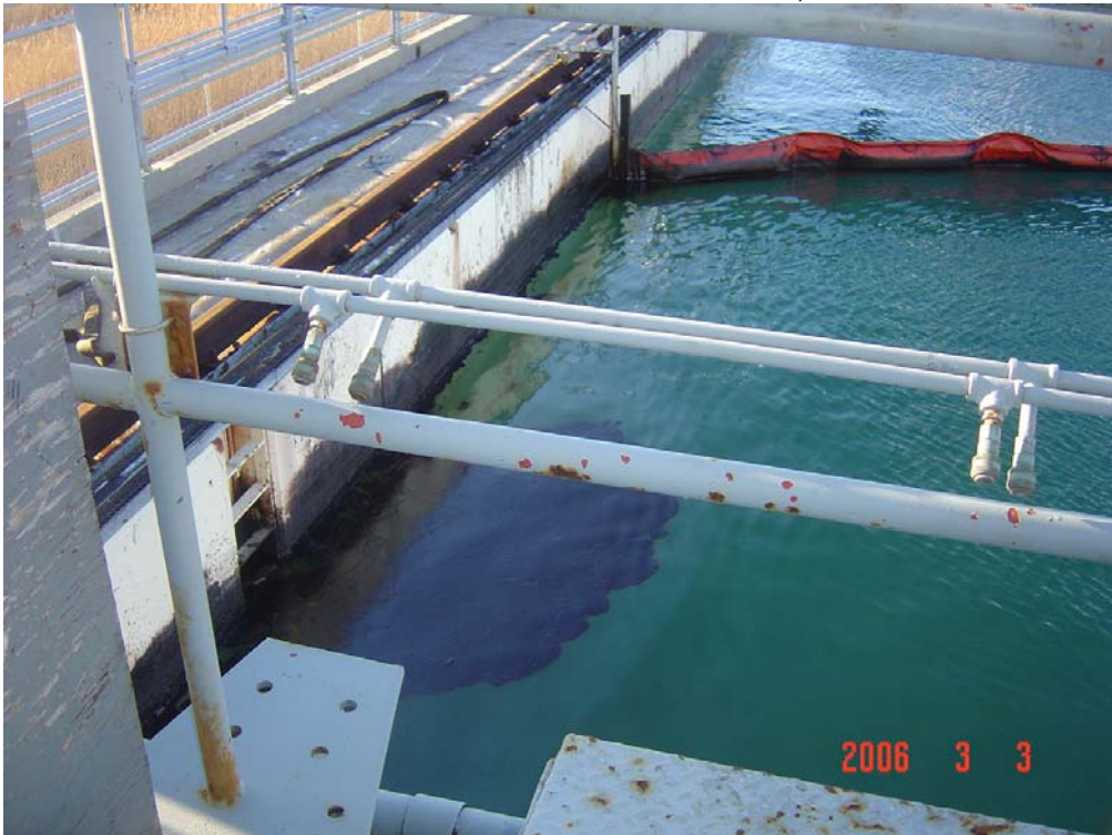
Figure 9: Accumulated oil in Ohmsett Test Tank from Dispersant Tests (photos taken 0730 on 3 March 2006, before Tests 10 and 11)
