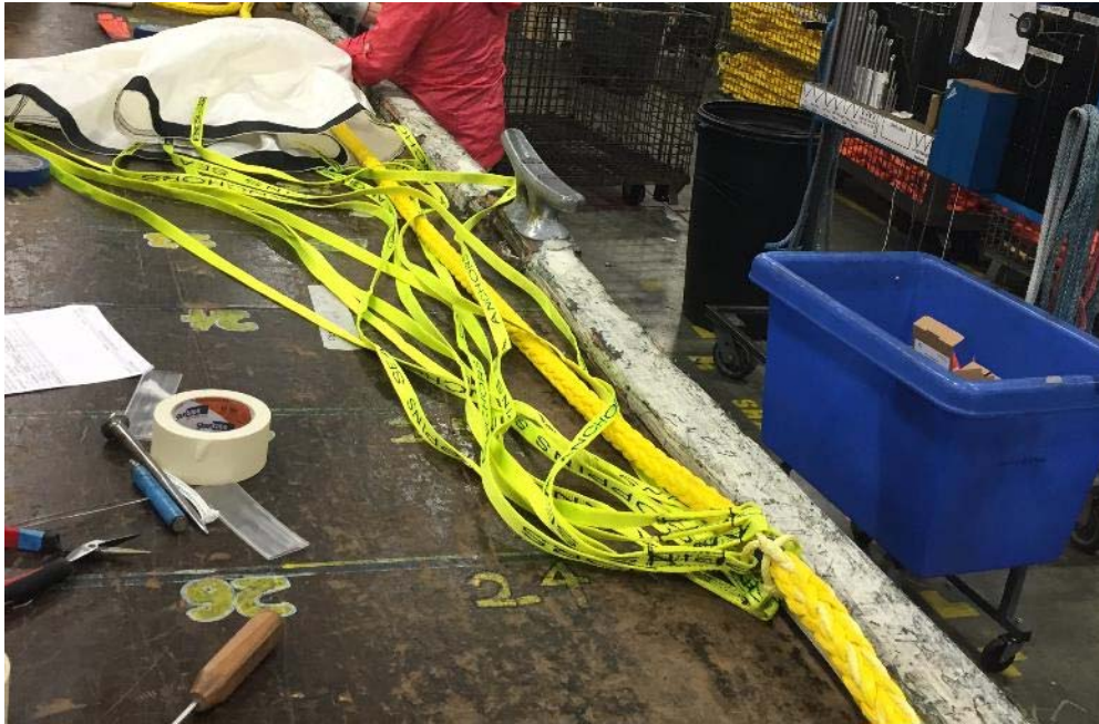
Figure 9 Photo of a Coppins Para Sea Anchor spliced onto the body of a floating retrieving line at the Samson Rope factory in Ferndale, WA
