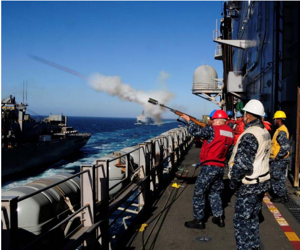
Figure 7 Photo of an impulse-projected type line-throwing device being discharged from the deck of a US Navy vessel; photo from survivalmonkey.com
