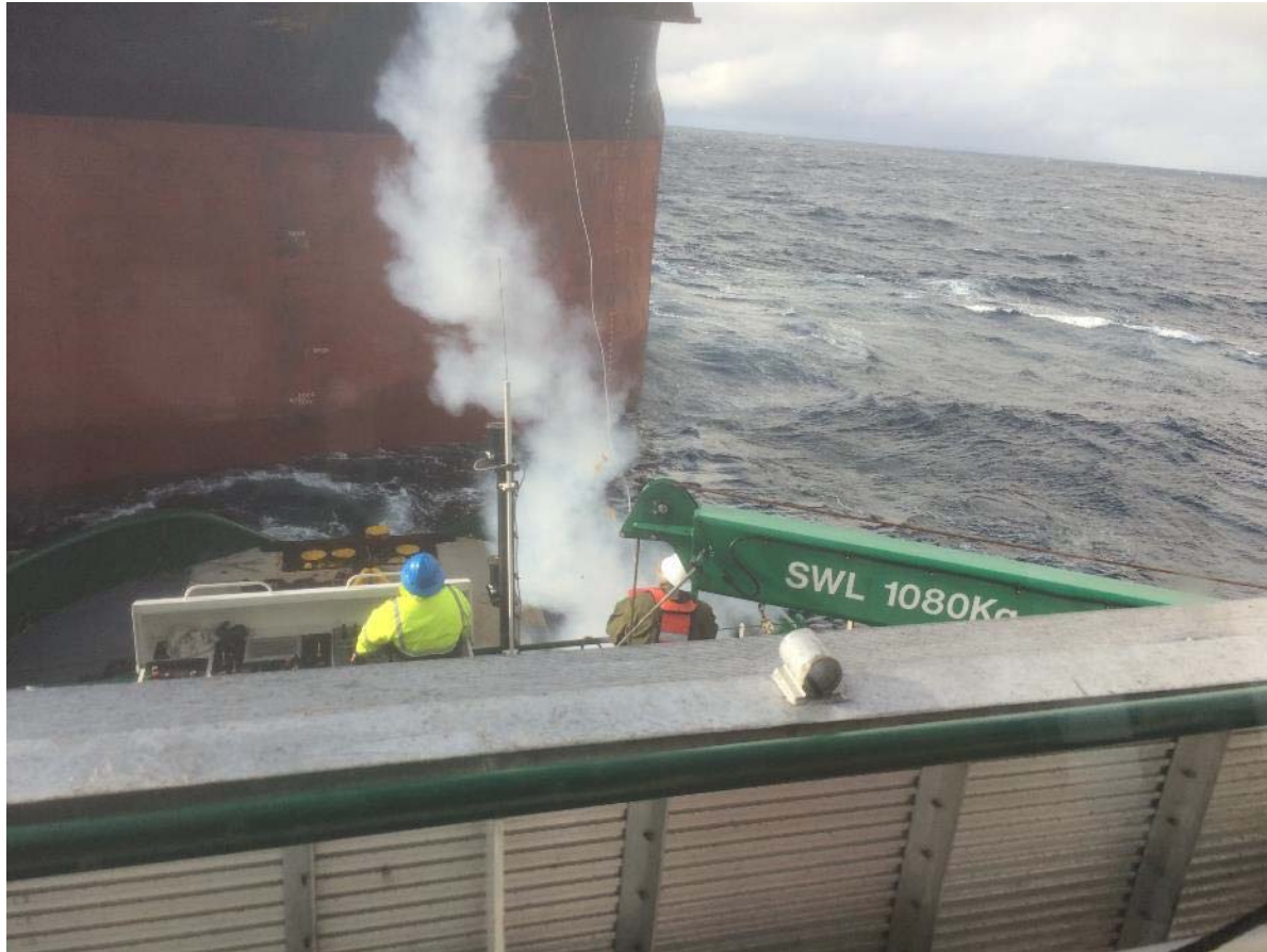
Figure 14 Photo of the initial (missed) shot from Michele Foss to Ecofaith G.O. , using a Pains-Wessex pyrotechnic type line-throwing device; photo courtesy of Foss Maritime
