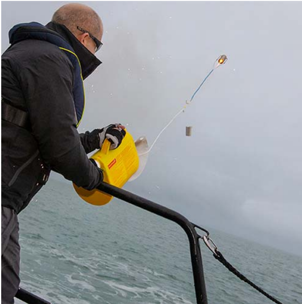
Figure 3 Photo of a pyrotechnic type line-throwing device being activated from the deck of a vessel at sea; photo from survivitecgroup.com
