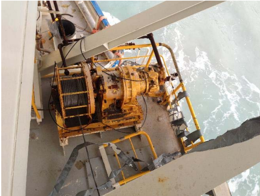
Figure 20 Deck mounted air tugger used to transfer the 10-inch Dyneema from the Aiviq to the Kulluk
