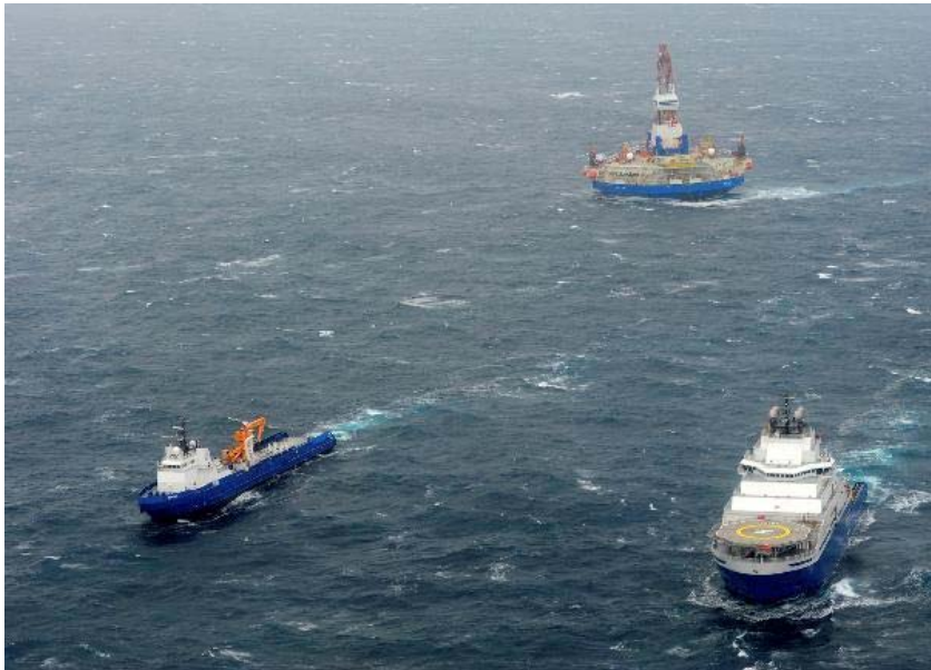
Figure 17 Kulluk under tow with both Aiviq and Nanuq connected; photo from Anchorage Daily News
