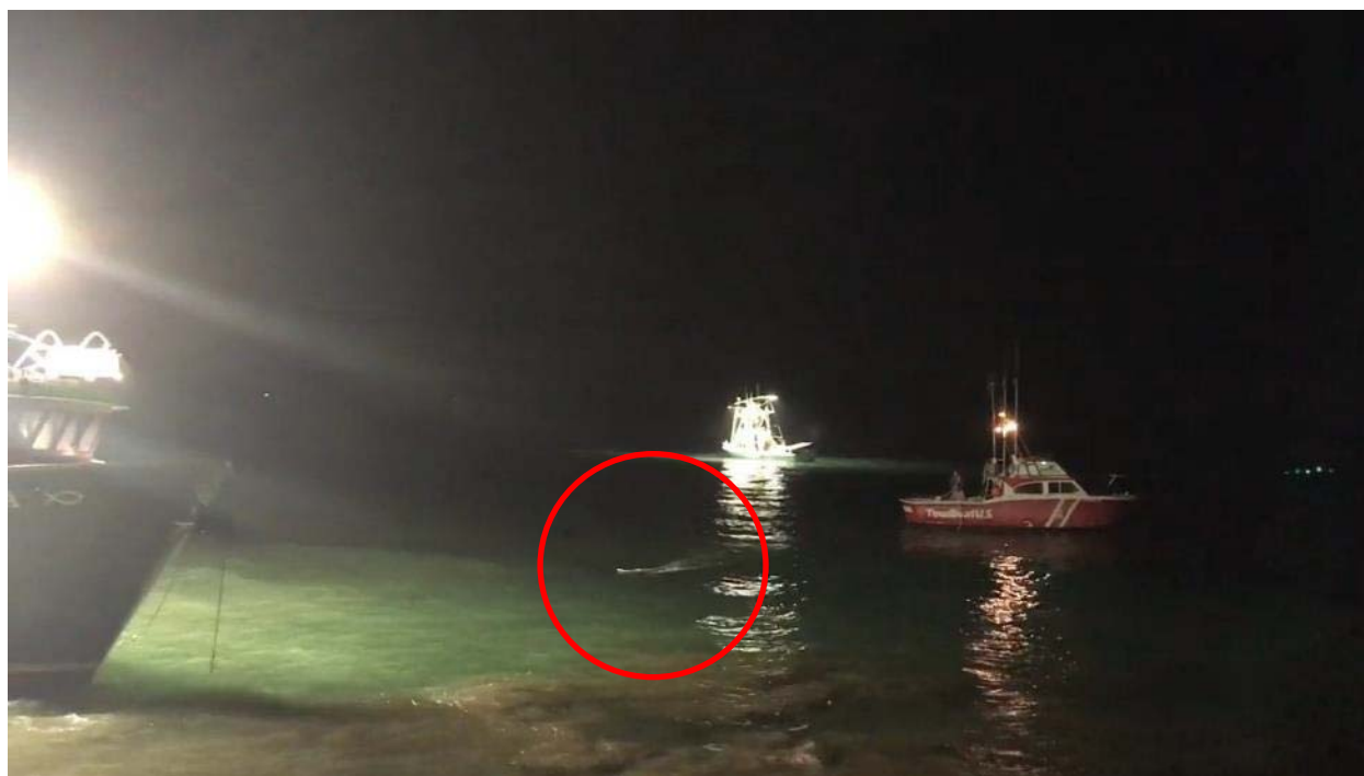
Figure 15 Image of a waterborne drone delivering a floating messenger line to the grounded fishing vessel, Emerald Sea (visible inside the red circle)
