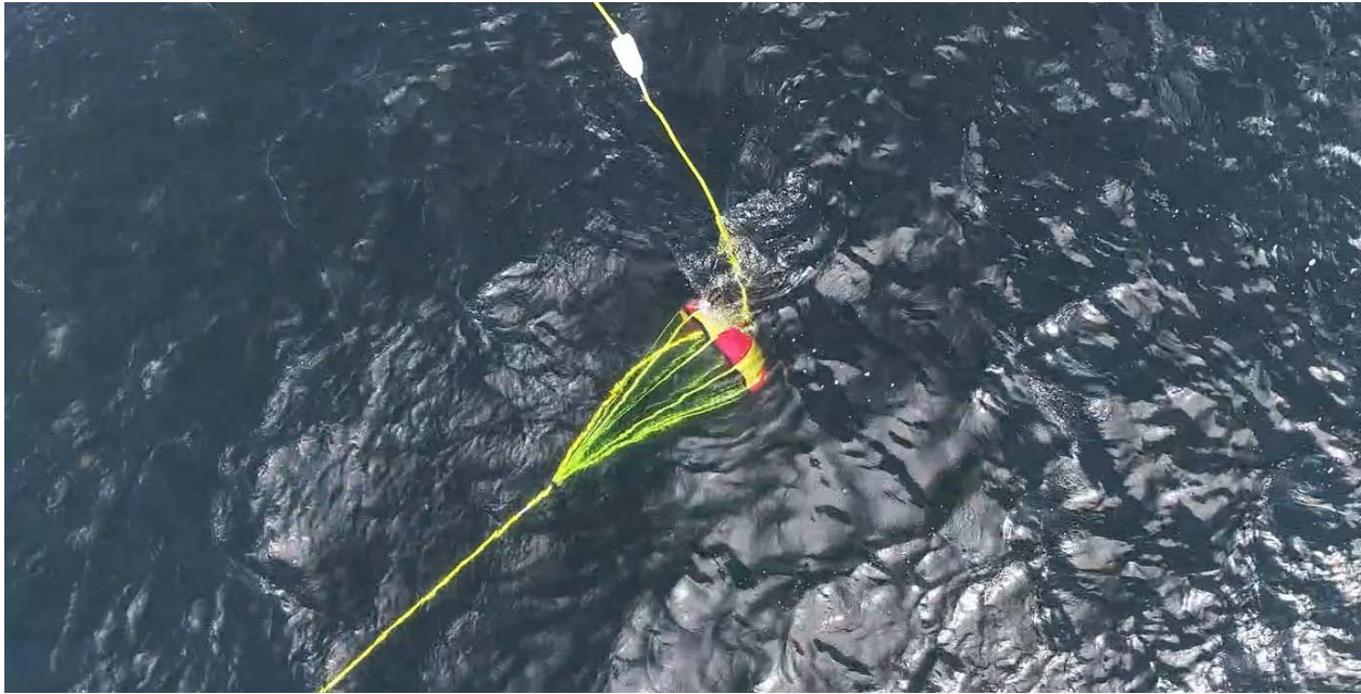
Figure 5 EVATS float line system after deployment
