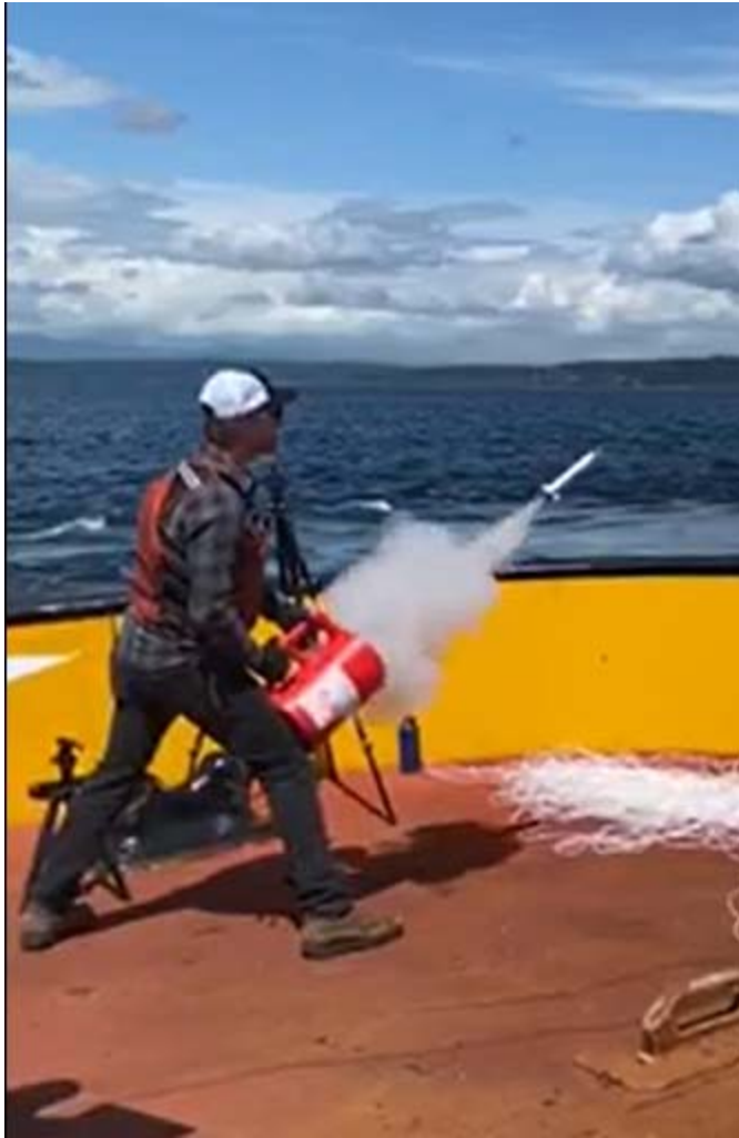
Figure 6 Ikaros Line Thrower deployment
