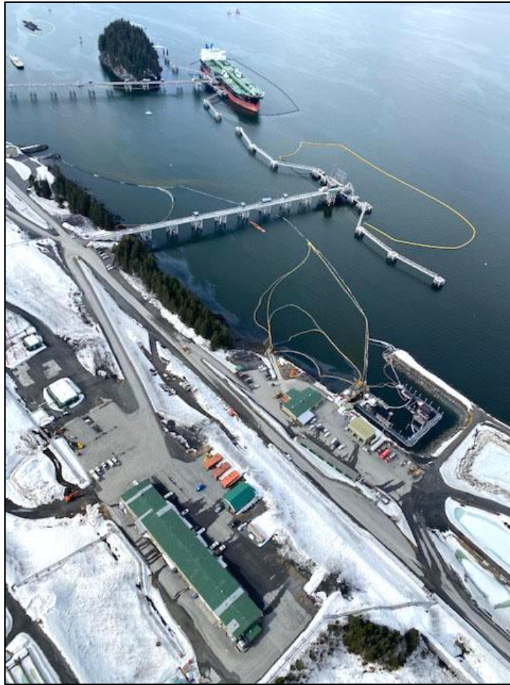
Figure 2. Containment booms placed around the spill site and in adjacent waters. Saw Island in upper left background adjacent Berth 5 tanker. Image from Alyeska Pipeline Service Company.
