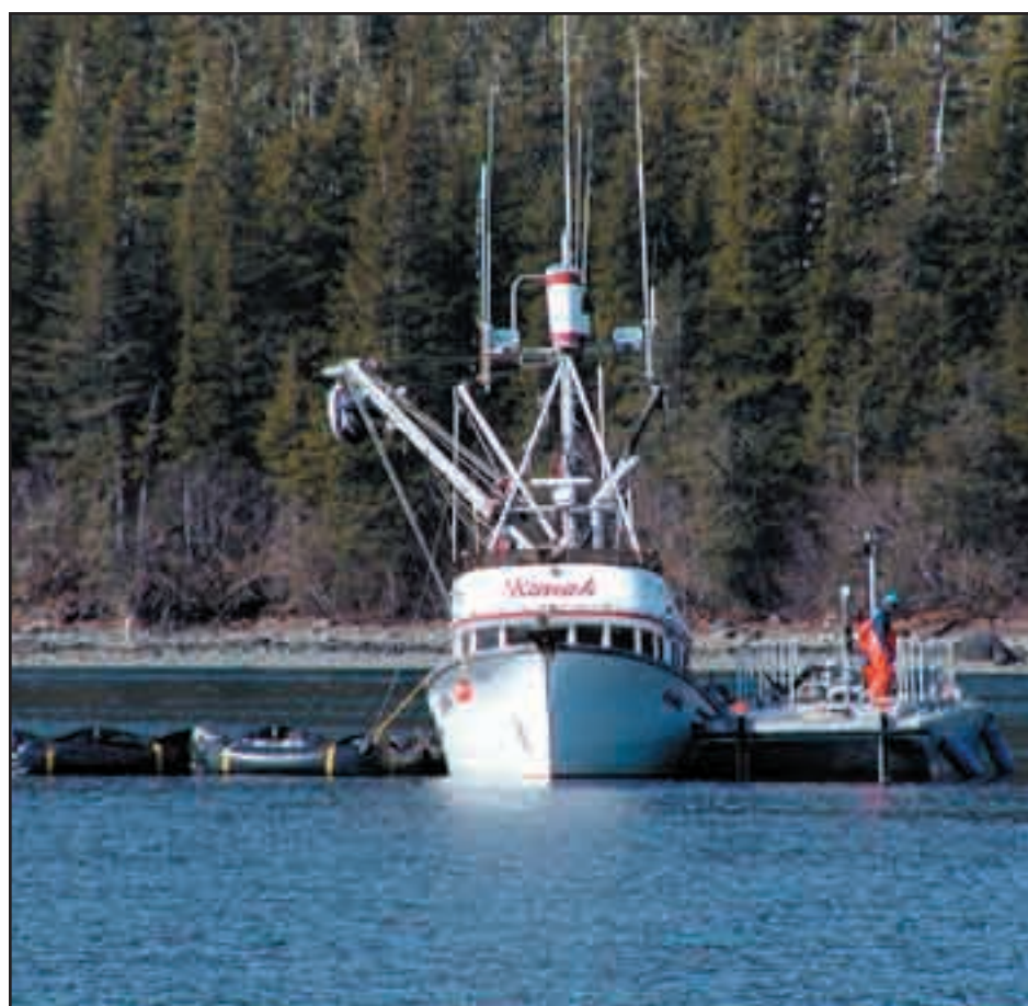
Port Fidalgo (near the village of Tatitlek) was the scene of an April 25 drill testing nearshore response capabilities. Here, in Landlocked Bay, crew members of the fishing vessel Kanak work on a minibarge as a skimmer collects "oil" from within containment boom and pumps it via hose over the Kanak's deck to the barge. Photo by Joe Banta.
