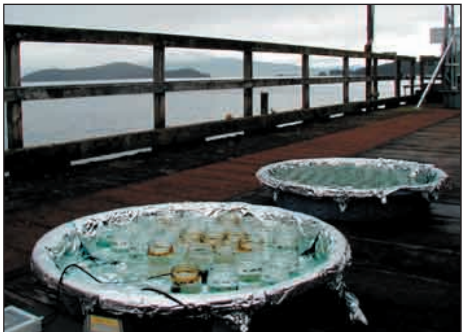
RESEARCH -- The council's phototoxicity study was conducted at the Auke Bay laboratory (above), near Juneau. Below, herring samples are exposed to sunlight to test whether it increases the toxicity of North Slope crude oil in seawater. Photos courtesy of Dr. Mace Barron.
