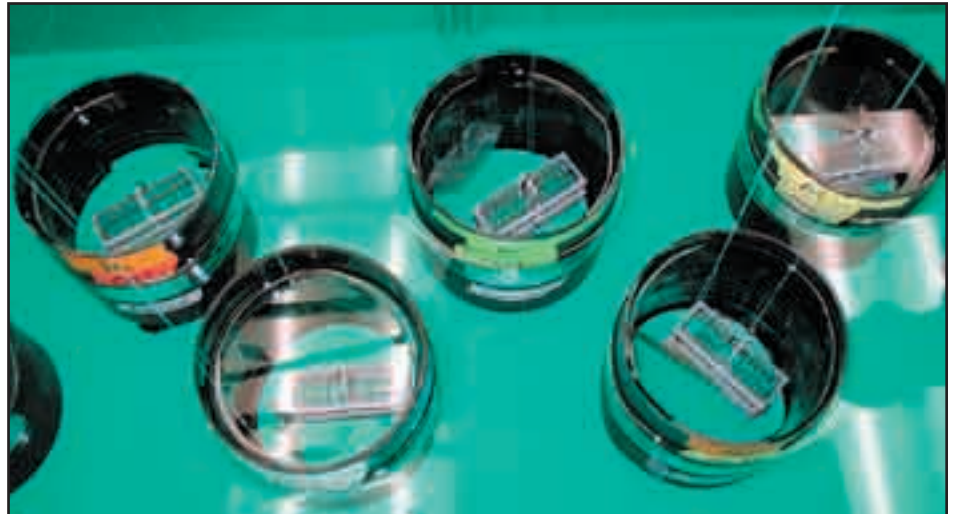
This apparatus was used to expose herring eggs to North Slope crude oil in the council-sponsored phototoxicity study. Photo courtesy of Dr. Mace Barron.
